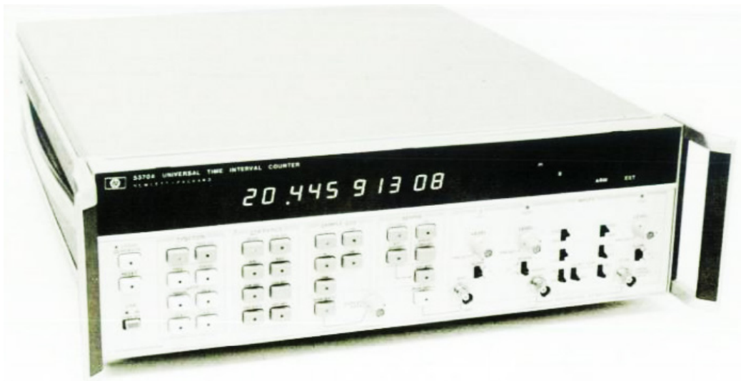
Fig. 2.1 HP 5370A universal time interval counter with 20-ps resolution, 10 seconds range and frequency up to 100 MHz.
