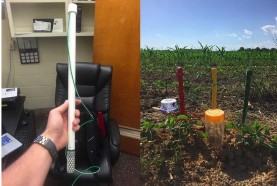
Figure 6. Completed matric potential sensor with attached Watermark sensor. Sensors were placed at 20, 40, and 60cm depths during both growing seasons.
