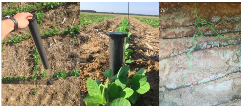
Figure 5. Full view of minirhizotron tube prior to installation, minirhizotron tube installed at 90-degrees within soybean row, and manually tracing collected image in Rootsnap software.
