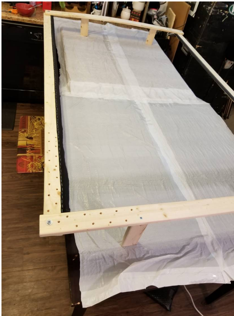
Figure 23. Wooden frame with added legs.
