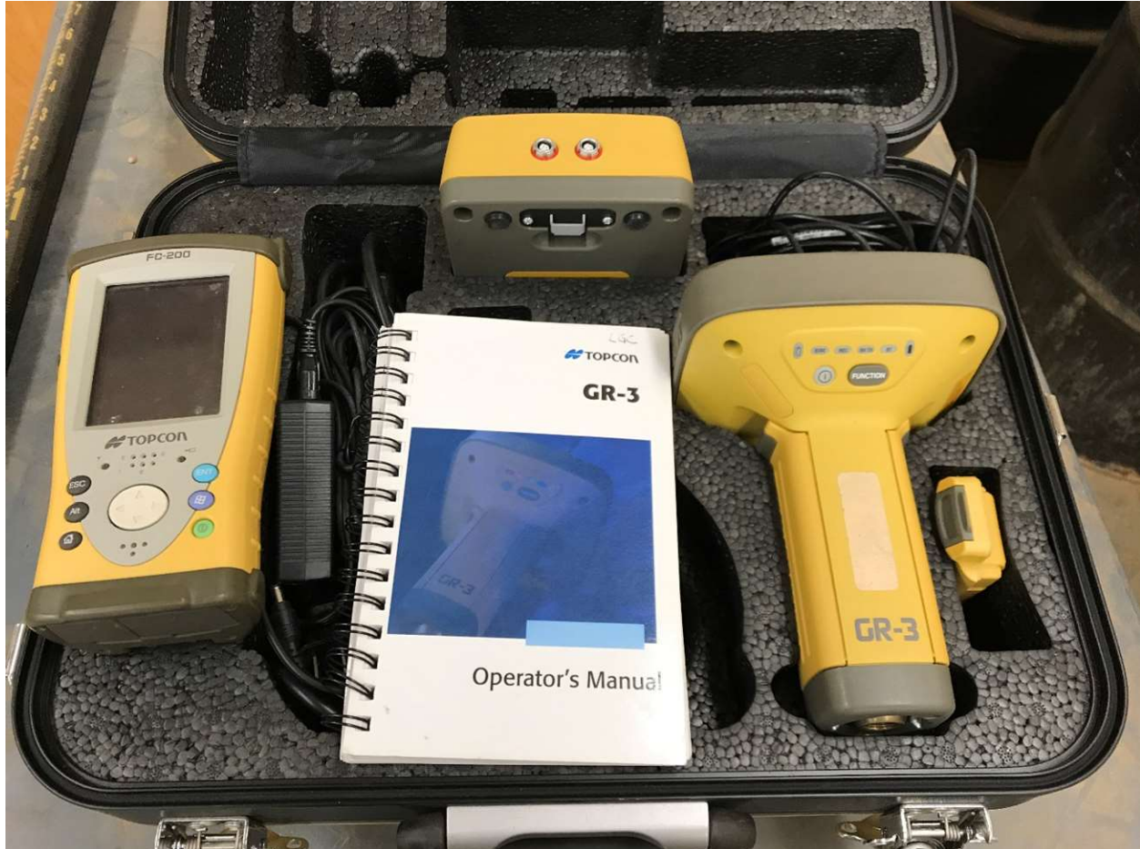
Figure 20. GR-3™ GPS receiver, Topcon FC-200 and operator's manual for survey (Topcon Positioning Systems, Inc.).
