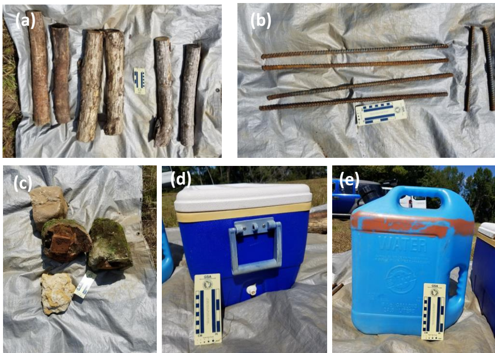
Figure 9. Images of the specific objects buried at EV Smith Research Center including: (a) six logs, (b) four of six pieces of rebar, (c) two rocks and two blocks of cement, (d) a rectangular cooler, and (e) a 6 liter carboy.
