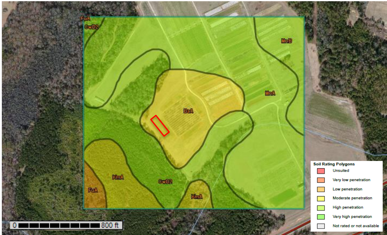
Figure 8. Soil map generated by Web Soil Survey (USDA NRCS, 2017) showing suitability of GPR for different soil types based on texture, composition and slope.
