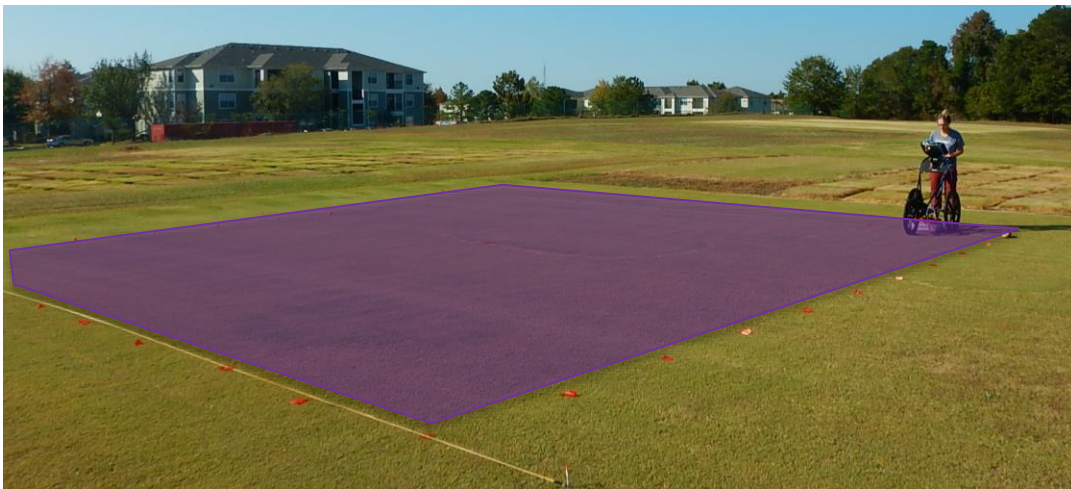
Figure 11. Image of GPR data acquisition on turf plot. Purple box indicates area of 10 m x 10 m grid and orange flags are markers for 1 m spacing.
