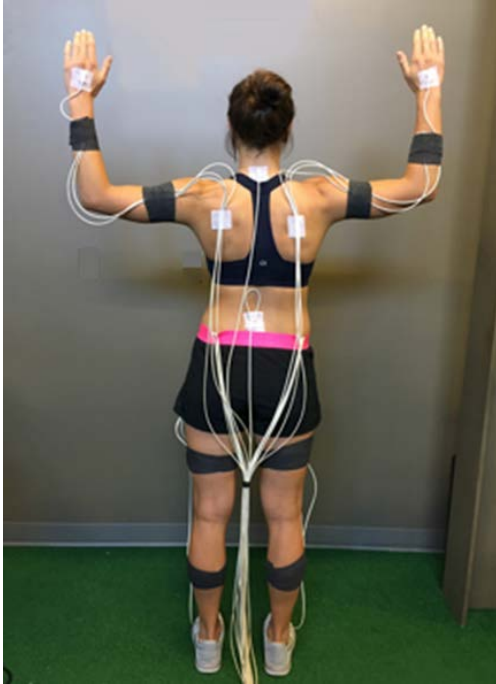
Figure 8. Electromagnetic sensor attachment.
