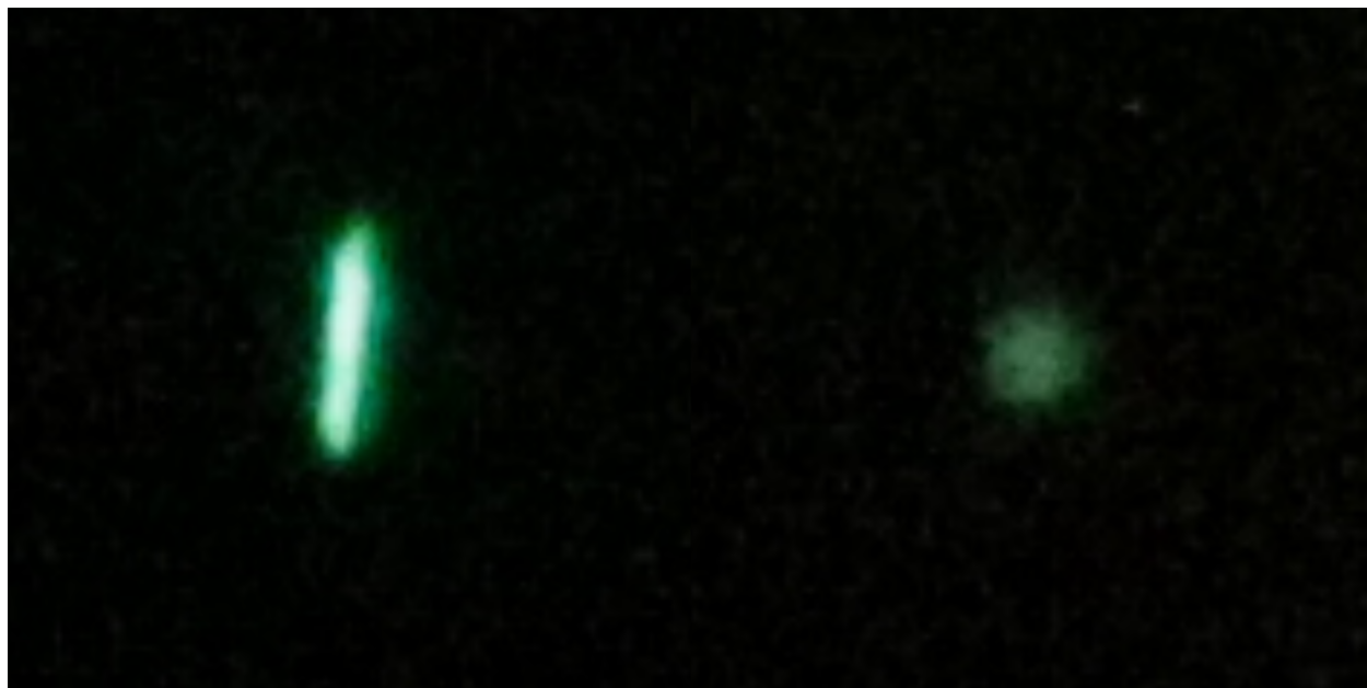
Figure 3.15: Typical high resolution photographs used for alignment. Left image: laser focus on phosphor. Right image: ALS spot at 18.44eV energy. To show more detail, the images have been clipped and expanded around the light spots.
