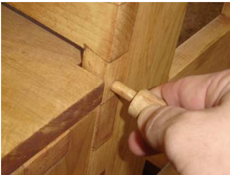
3. Insert peg to hold bench in front of desk.
