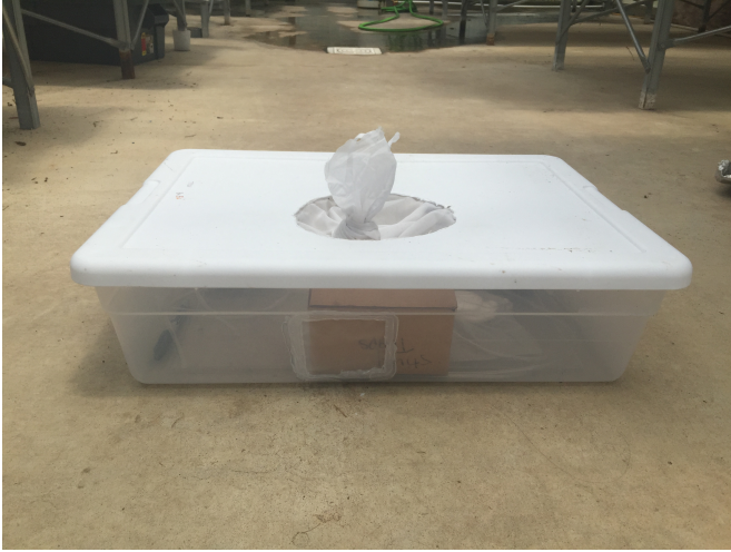
Figure 2.1. Inoculation access period cages modified to enable controlled whitefly release and provide air flow to contents.
