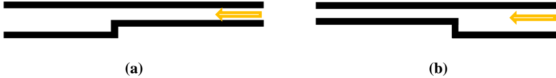
Figure 1.20 Schematic of the step geometries: (a) backward-facing step, (b) forward-facing step
