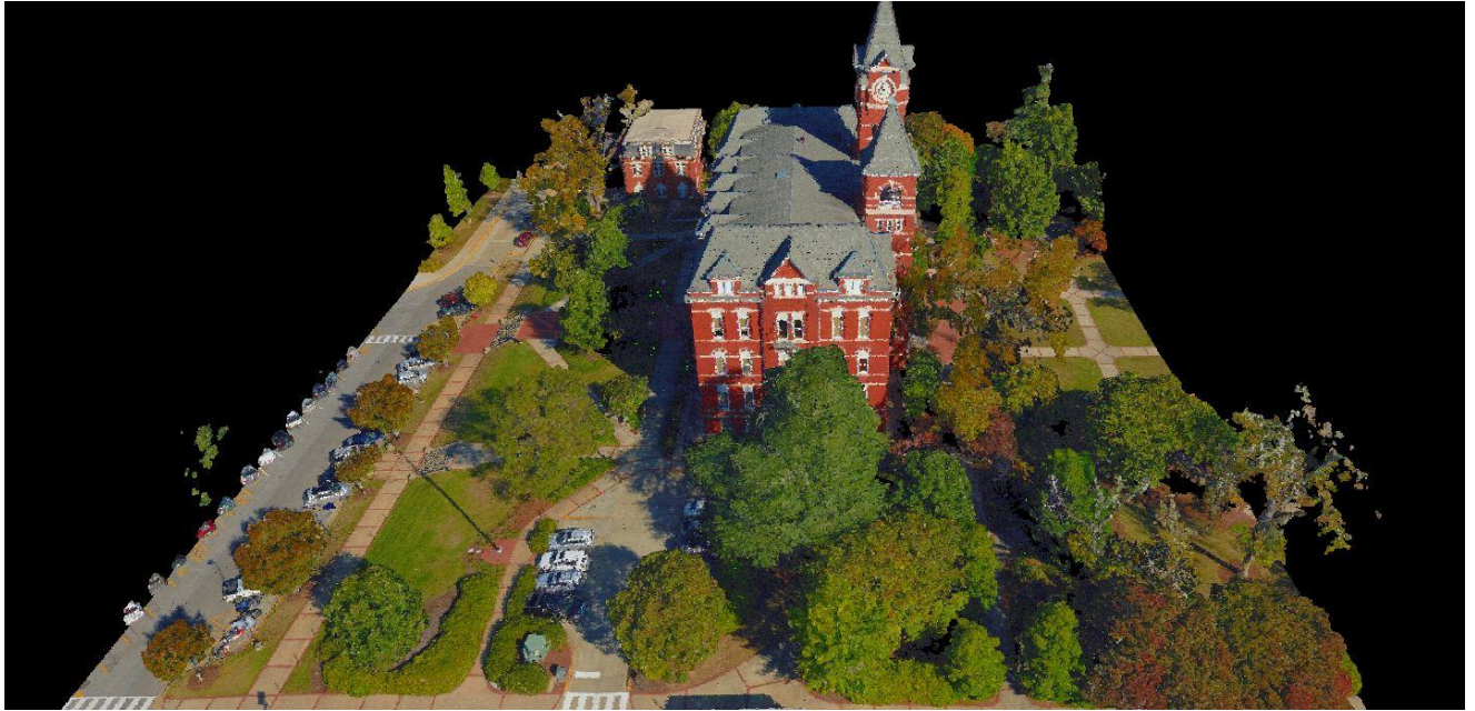
Figure 4.4 Portion of the study area shown using point cloud generated from oblique image viewers.
