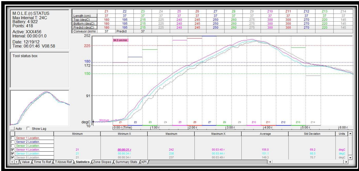
Figure 16 Lead-free Reflow Profile Bottom Side
