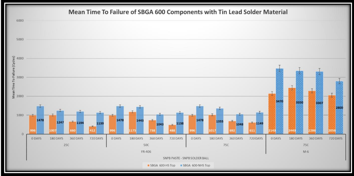
Figure 48 Mean-Time-To-Failure for SBGA 600 Components Tested with Tin-lead Solders
