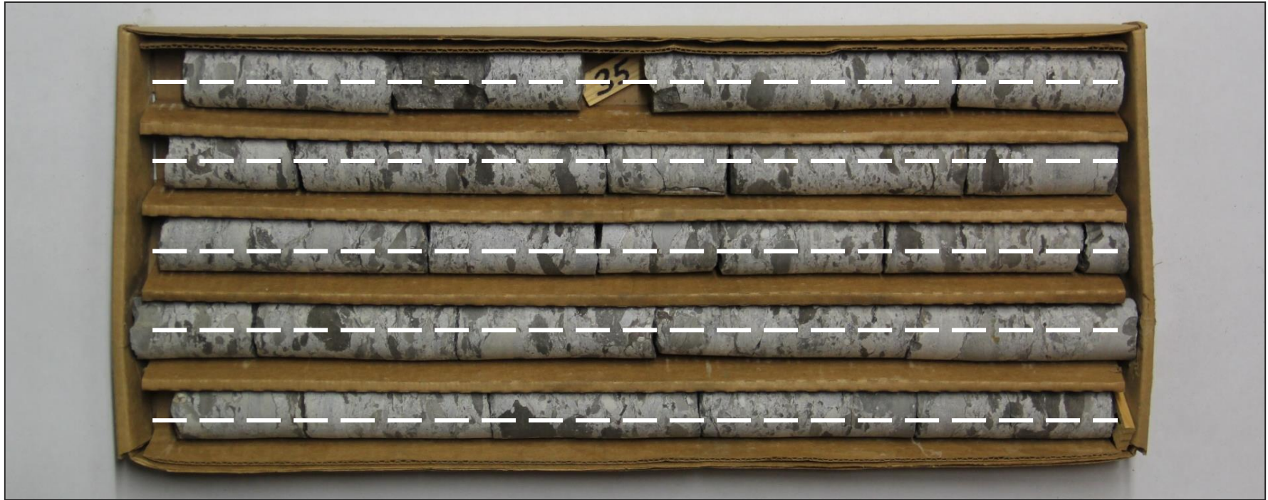
Figure 3. Flynn Creek drill core FC77-3, core box number 4, depth 10.7-13.7 m, which has been marked with dashed lines to simulate the location of a pencil line for the line-logging method. The length of each slot within the box is two English feet, or 61 cm.
