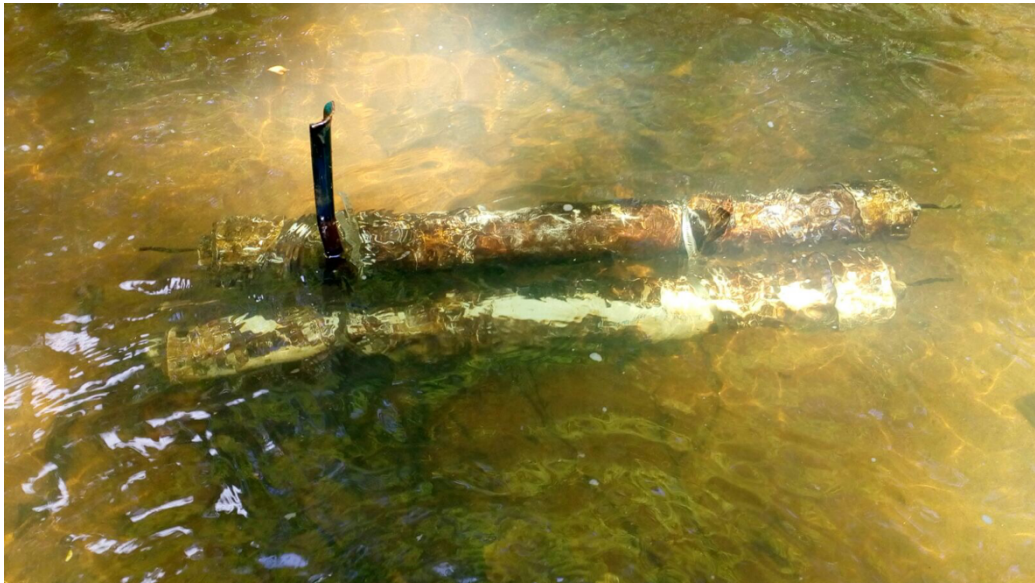
Fig. A4. Time integrated in-situ suspended sediment collection samplers
