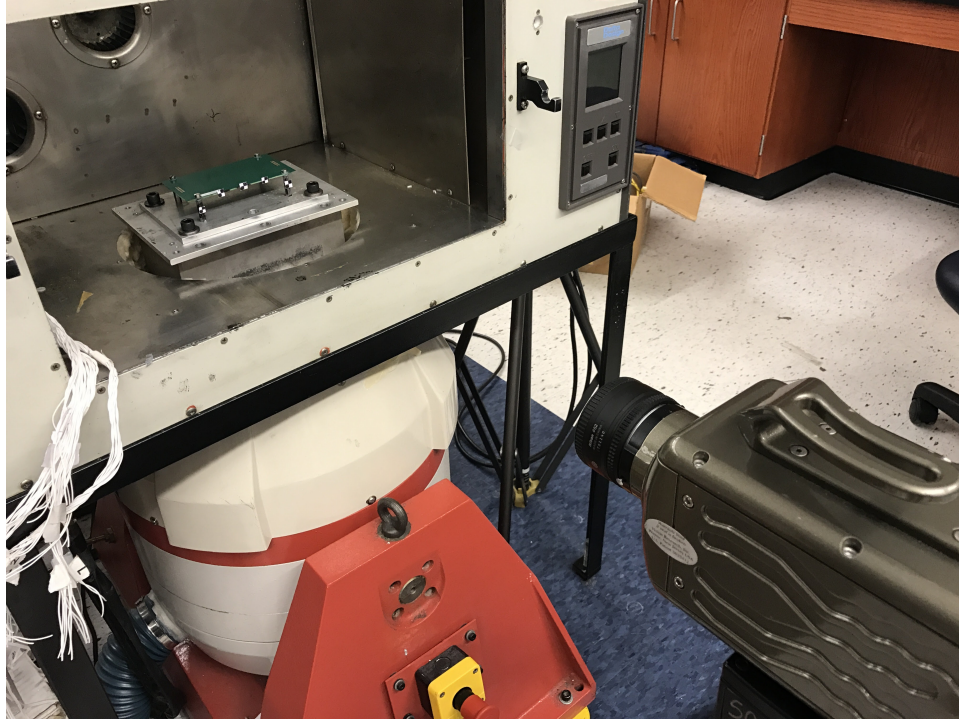
Figure 5.19: Experiment Setup of High Speed Camera
