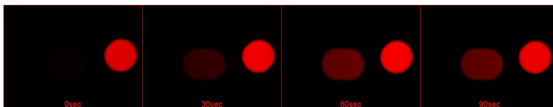
Figure 4.6: The progress of the detection kit’s enzyme reaction was monitored in static droplets. The smaller droplet was reference droplet with 85 \mu\text{M} resorufin, and the larger was the sample droplet containing 100 \mu\text{M} glycerol, enzymes, substrate, and ATP. Imaging started as soon as the droplets were formed. The produced fluorogenic molecule, resorufin, in the static sample droplet reached its highest concentration within about one minute
