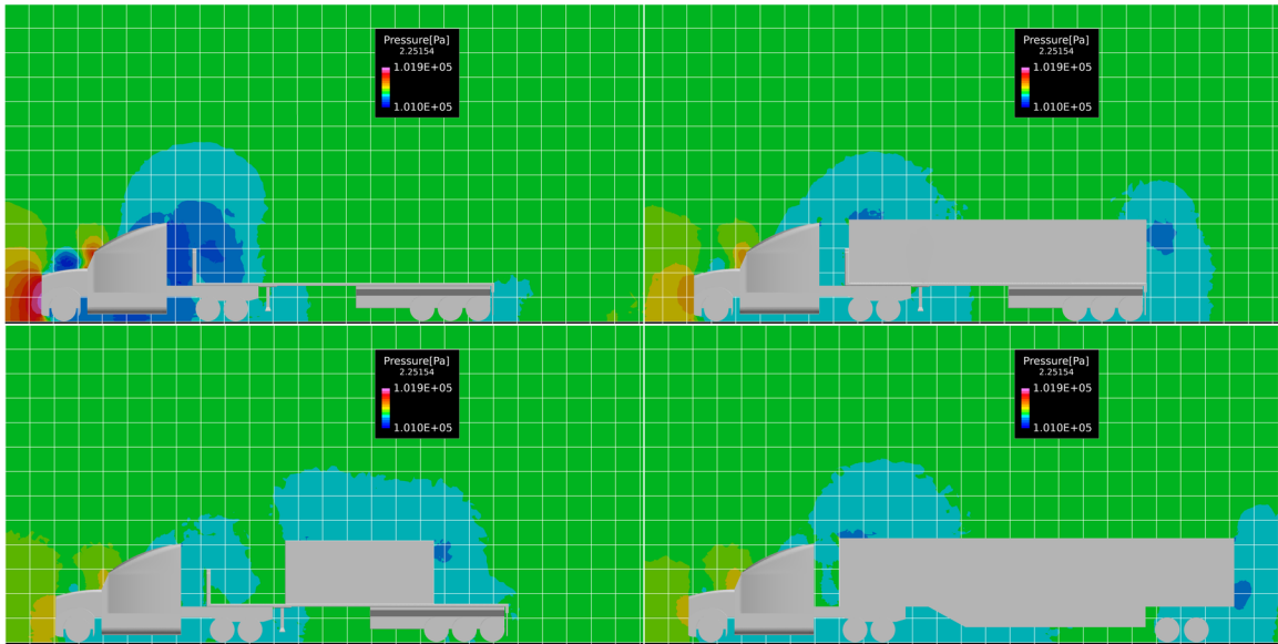
Figure 4.29: Static pressure contours for scenario 2, described in Table 3.3, at 50 ft.
