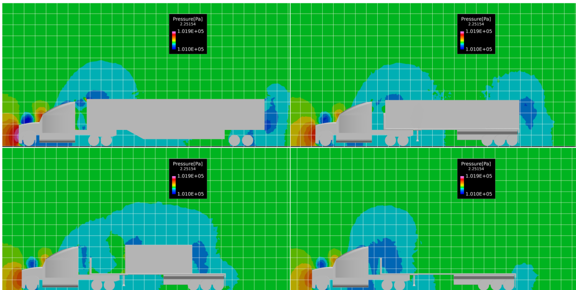
Figure 4.28: Static pressure contours for scenario 1, described in Table 3.3, at 200 ft.
