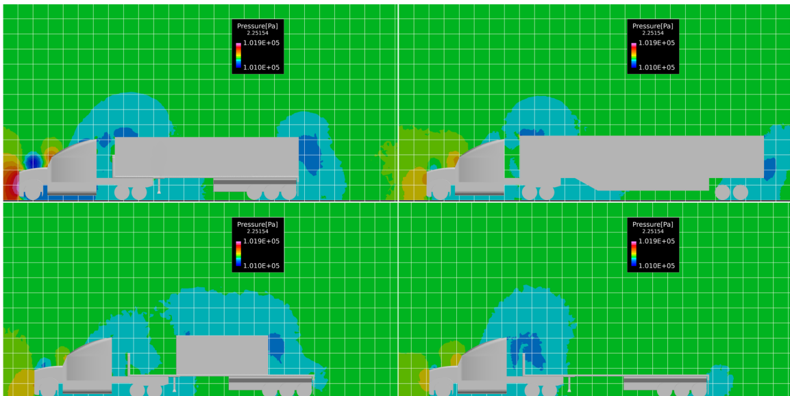
Figure 4.32: Static pressure contours for scenario 3, described in Table 3.3, at 50 ft.
