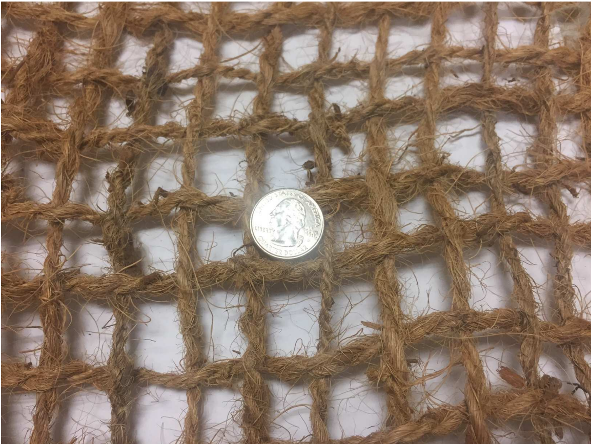
Figure 6.7: Single layer of jute/coir baffles used in experimental research of sediment basin flows
