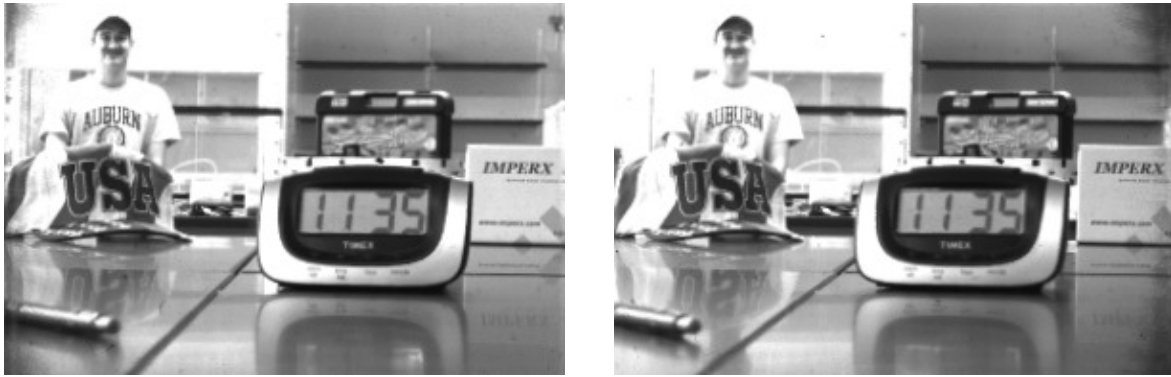
Figure 3.2: Computationally rendered image where the viewpoint of the observer has been changed to ( left ) the left side of the aperture and ( right ) the right side of the aperture.
