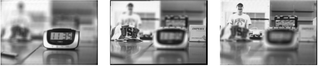
Figure 3.1: Computationally refocused images generated from a single exposure, focused: ( left ) on an alarm clock that is in front of the nominal focal plane, ( center ) at the nominal focal plane, and ( right ) on a student behind the nominal focal plane.
