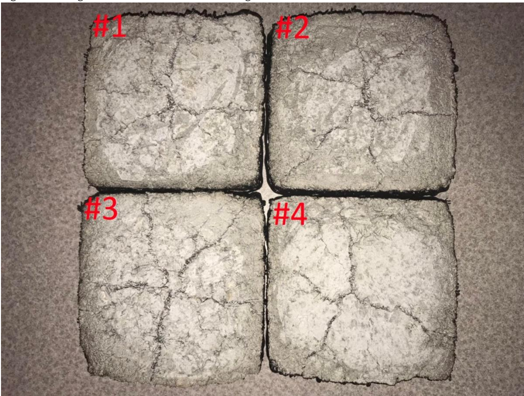
Figure 82 Image of concrete tiles after testing on the uncoated side
