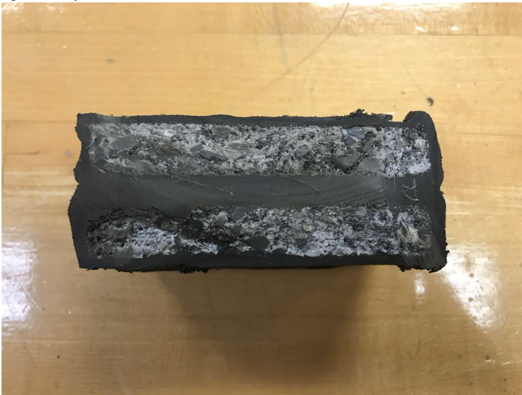
Figure 39 Polyurea coated on two sides of concrete
