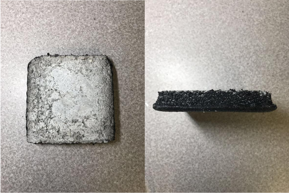
Figure 82 Image of concrete tiles after testing on the uncoated side
