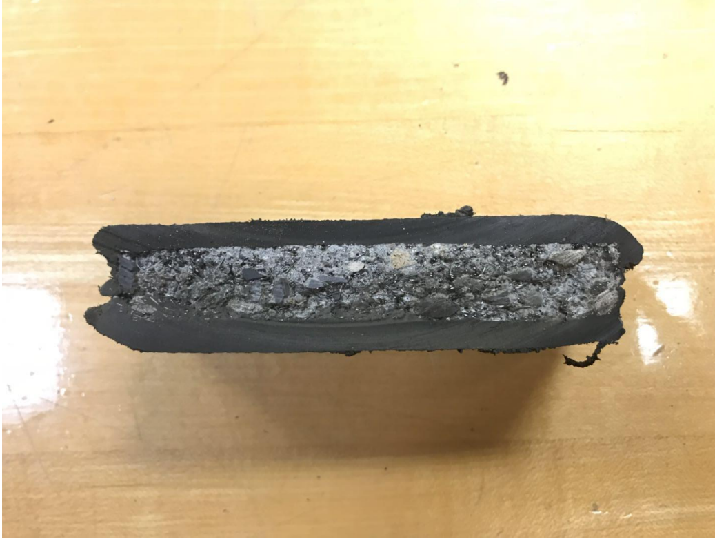
Figure 39 Polyurea coated on two sides of concrete
