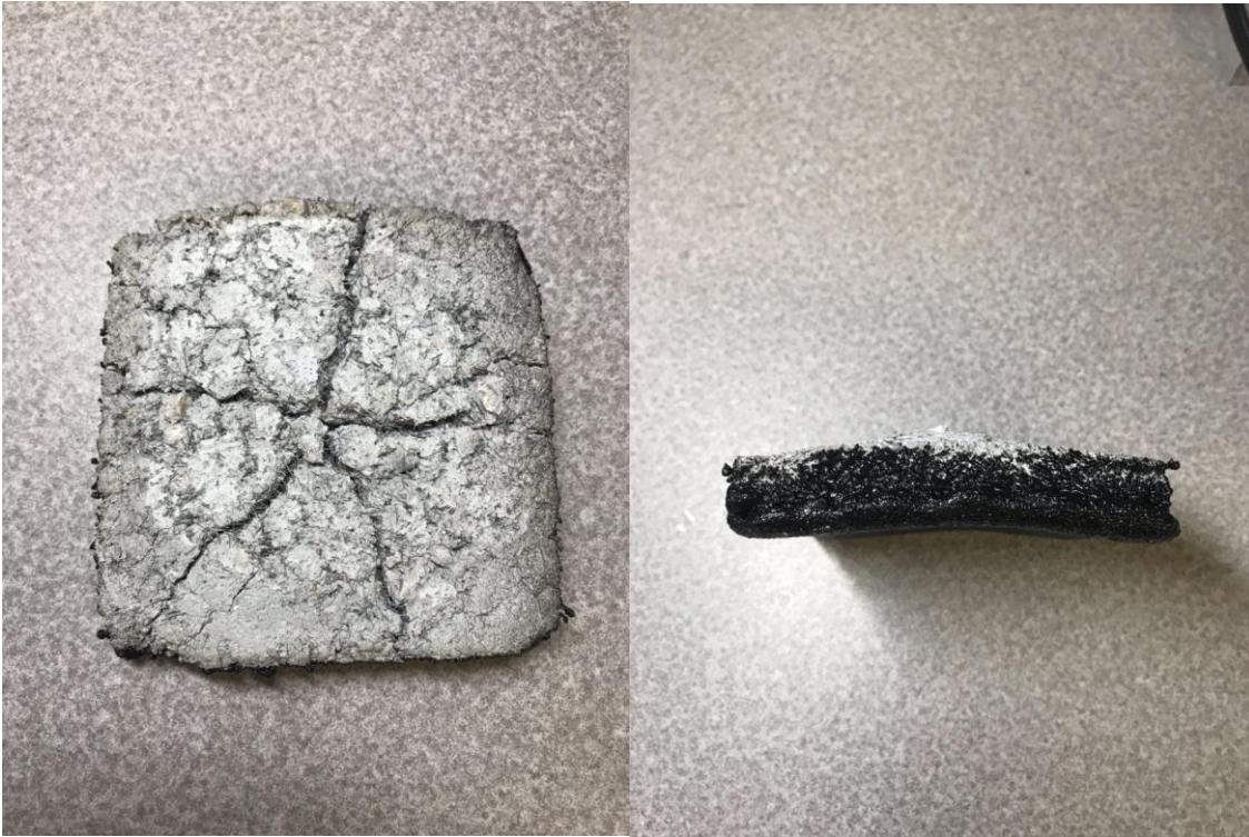
Figure 81 Image of concrete tiles after testing on the coated side
