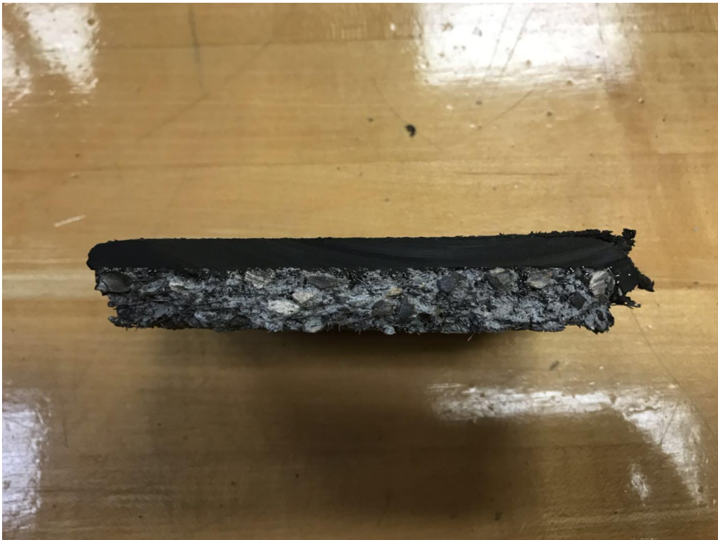
Figure 38 Polyurea coated on one side of concrete
