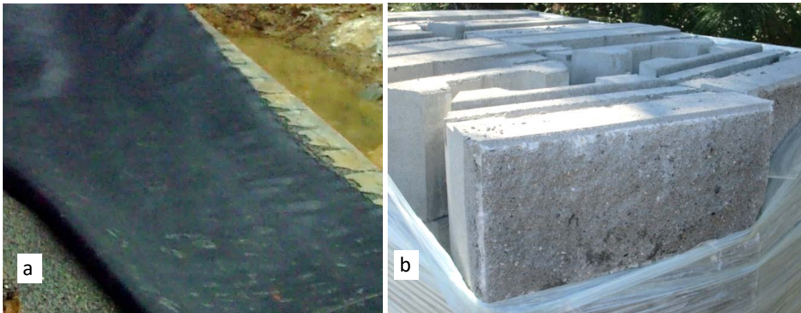
Figure 17. (a) Selected woven geosynthetic; (b) segmental retaining wall masonry units.
