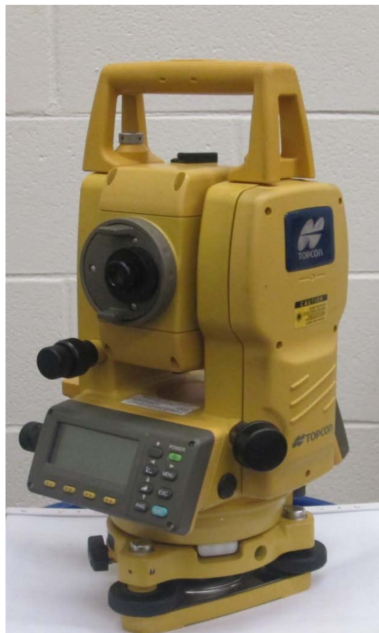
Figure 35: Topcon GTS-235W total station
