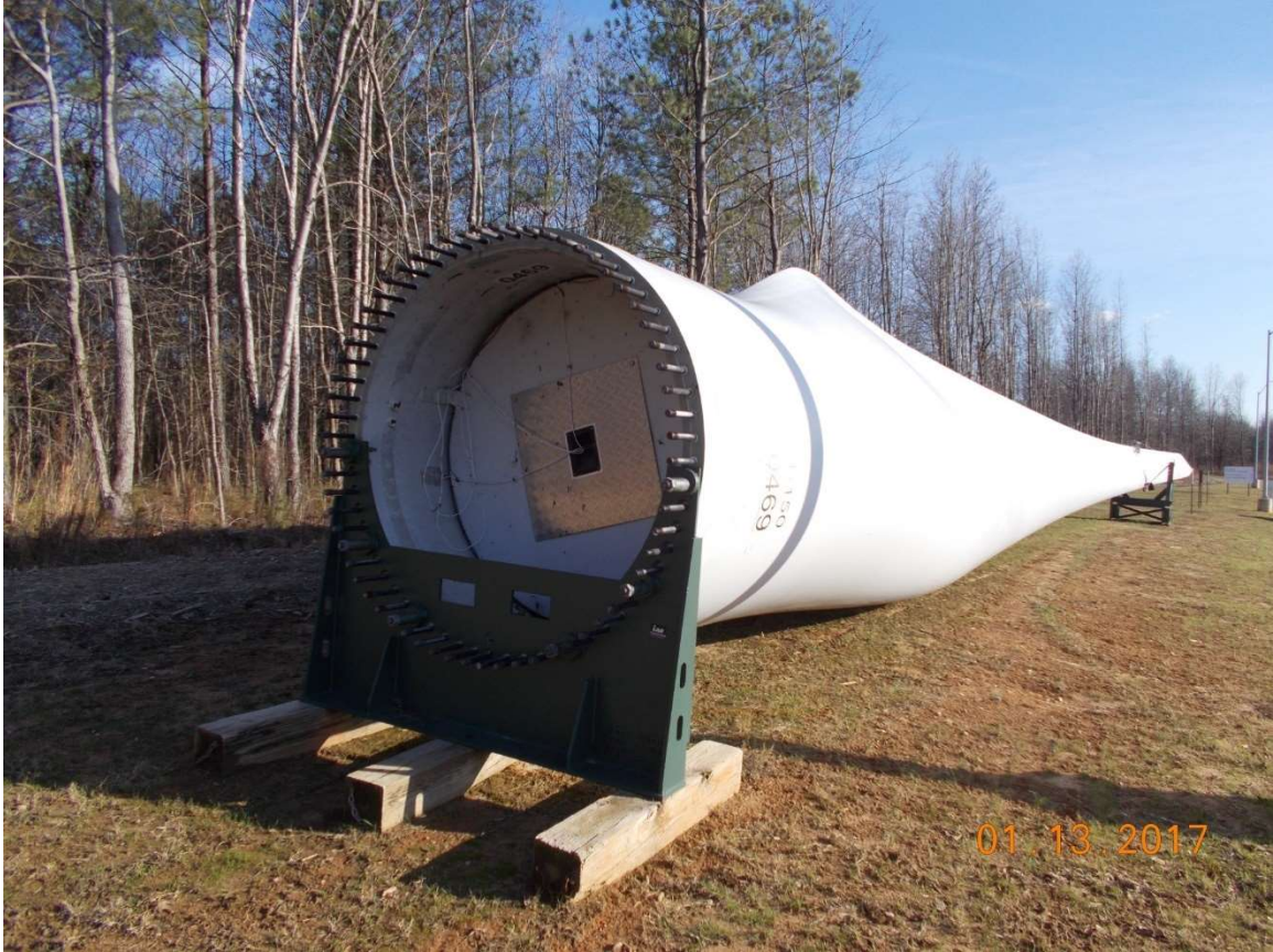
Fig. 2.3: A 40-meter wind turbine blade (photo taken by C. Bugg)
