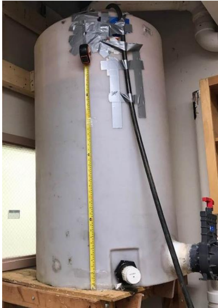
Figure 4. 8: The reservoir at the upstream of the pipe, with the 102-mm knife gate valve installed at the base of the reservoir.
