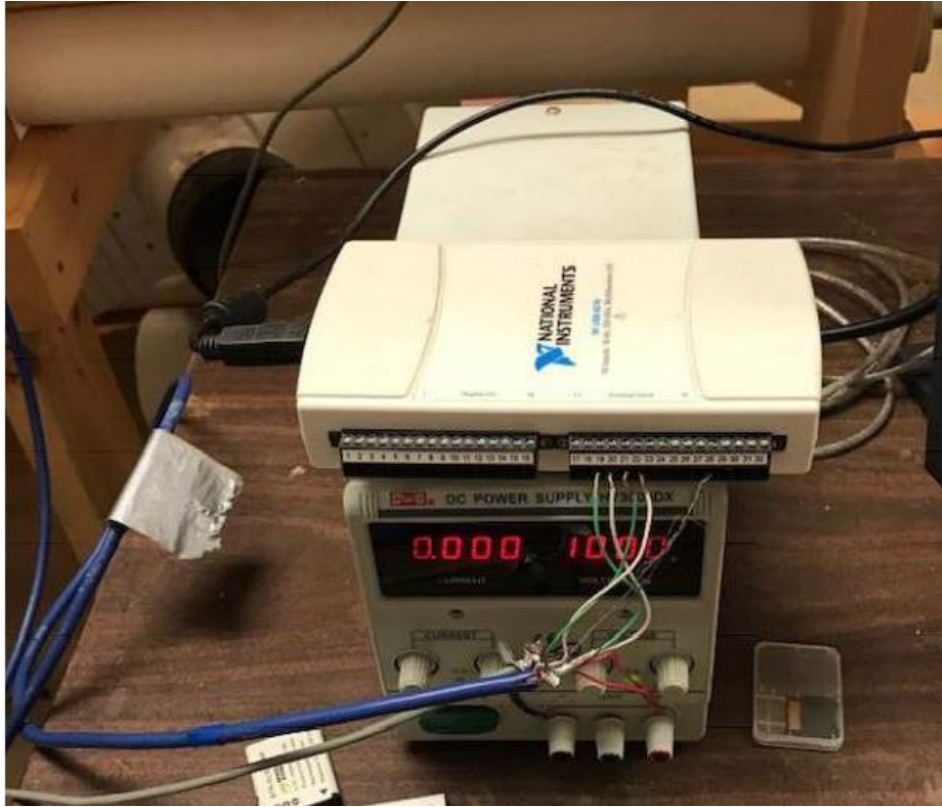
Figure 4. 6: Data acquisition board and its power supply.
