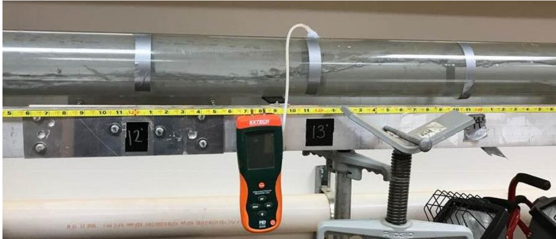
Figure 4. 4: Installation of manometer from the top of the pipe during the experiment.
