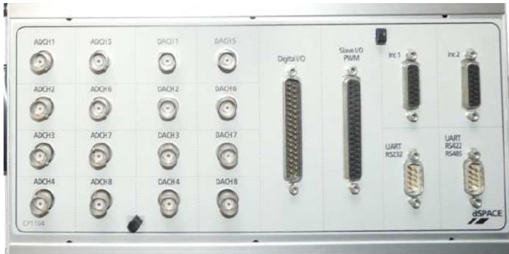
Figure 3.17: DS1104 R&D controller board.
