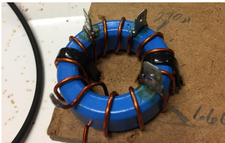
Figure 3.19: Adjustable inductor for the grid impedance.
