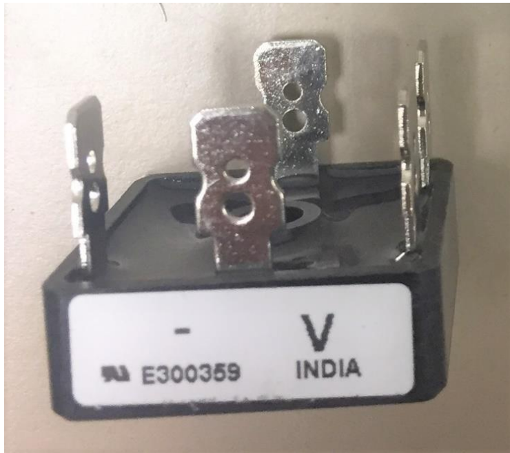
Figure 3.20: Three-phase diode-bridge rectifier.
