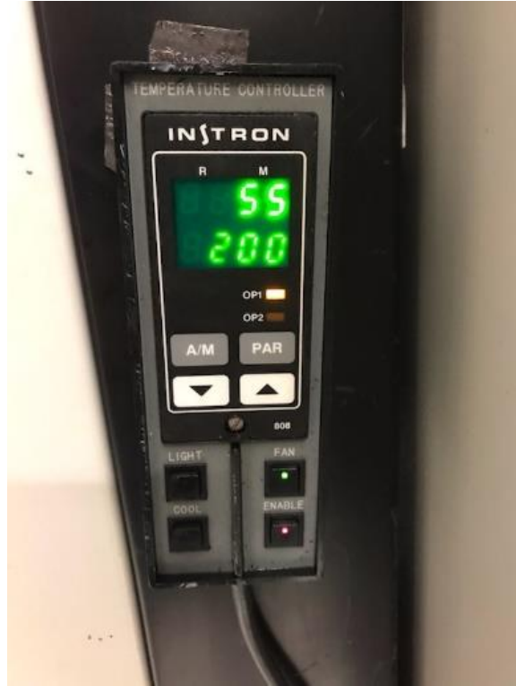
Figure 59: Thermal Chamber remote used to control the temperature inside of the chamber
