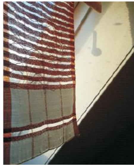
Figure 35: Interlaced SMA into Normal Fabric
