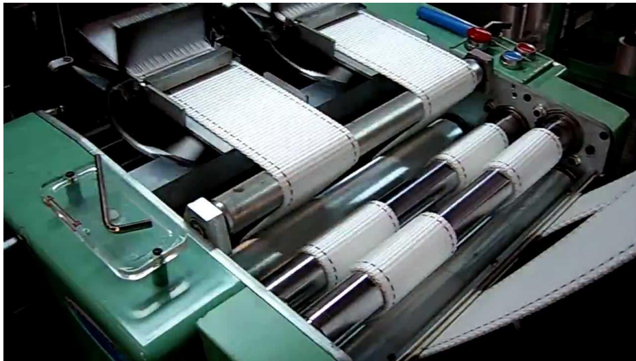
Figure 31: Fabric Take Up for a Narrow Fabric Weaving Machine [89]
