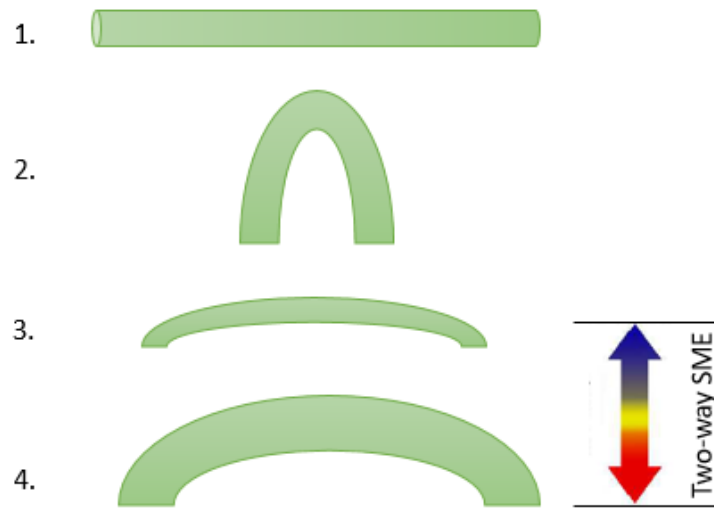
Figure 13: Two-way shape memory effect: (1) Martensite, (2) Deformation with an irreversible amount, (3) Heated, (4) Cool
