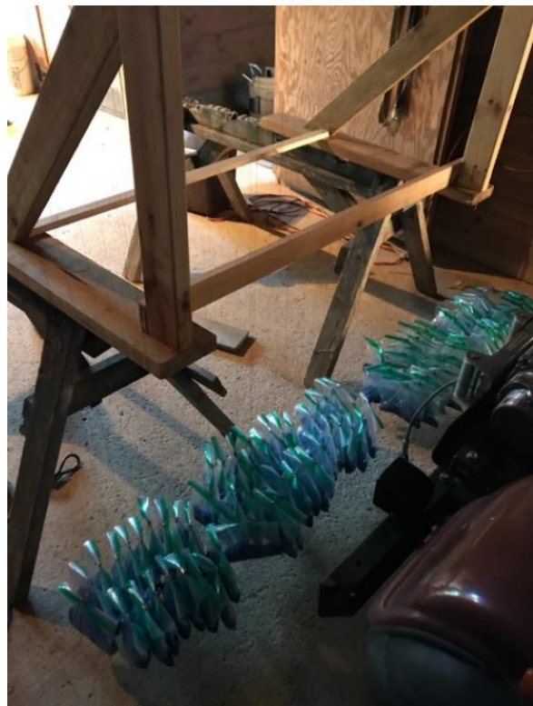
Figure 50: Individual Sandbags used to tension wires for Narrow Fabric Weaving Machine
