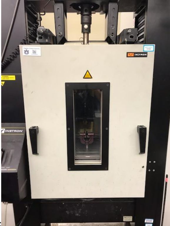
C Figure 58: Thermal Chamber attached to the tensile testing machine
