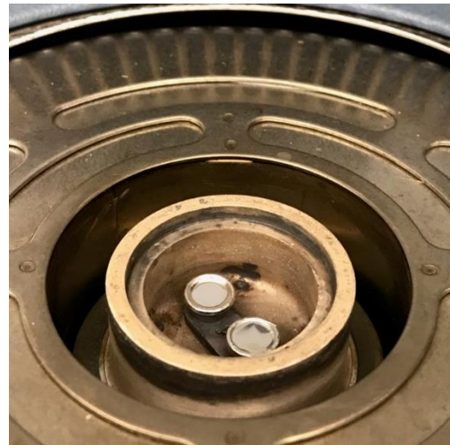
Figure 55: DSC sample and reference pan inside of testing chamber
