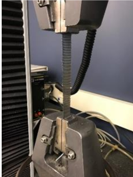
Figure 56: Woven Nitinol Fabric placed in jaws of tensile testing machine
