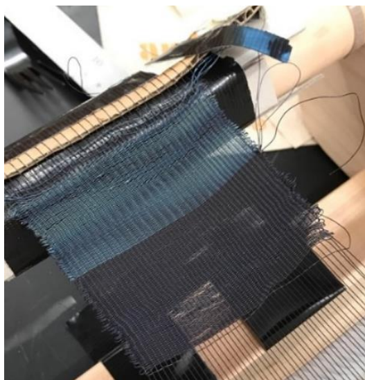
Figure 48: Hand woven fabric without binder cord
