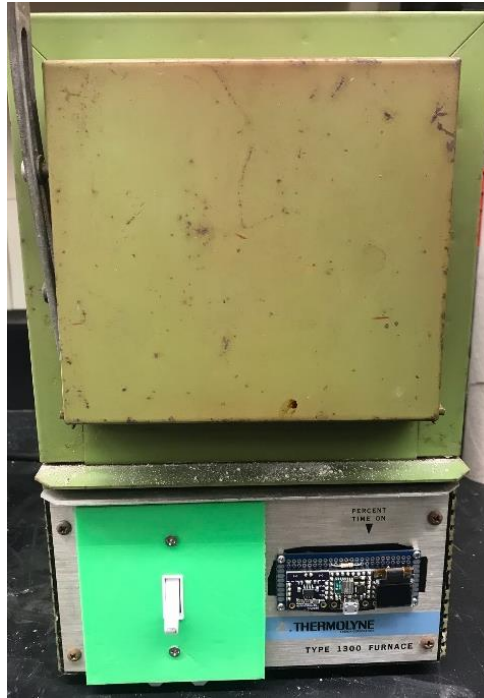
Figure 61: Furnace used to heat treat wire/fabric
