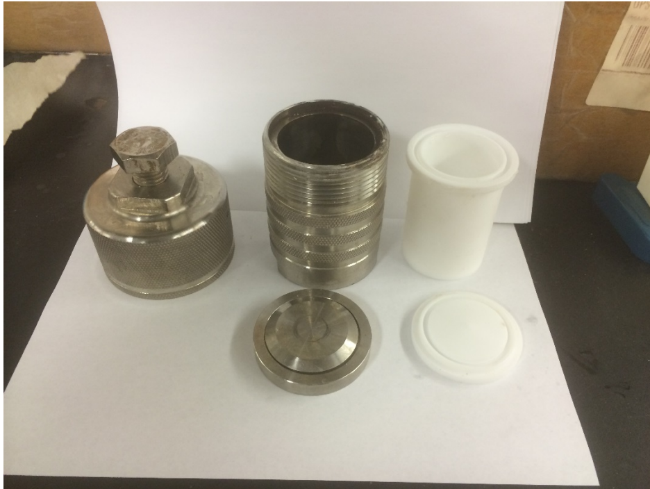
Figure A-3. Stainless steel jacket with a Teflon reactor for titanate nanotubes synthesis.
