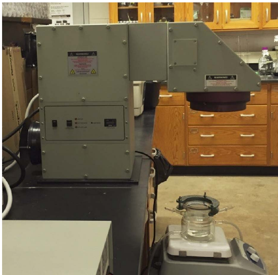
Figure A-2. A simulated photodegradation system. The arc lamp power supply can supply 450-1000 W power. The light source is a 450 W xenon-zone free short arc lamp with an air mass filter. The optical path area is 4 \times 4 inch.
