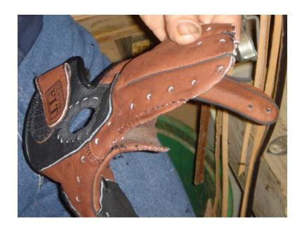
Figure 41- Construction: Finger Structure Removed
