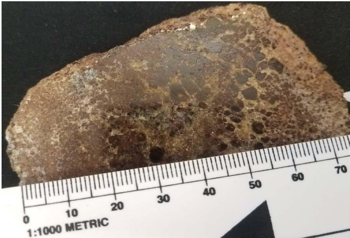
Figure 17 - Cut and polished slab sample (65.3B) of garnetite from the Waresville Schist. It typically appears as a nearly uniform massive reddish brown rock, as in the top left part of this sample.
