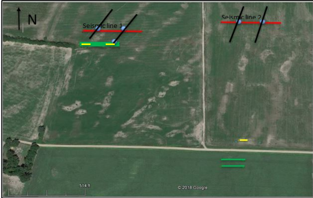
Figure 28: Pritchett site map showing location of seismic reflection surveys (red lines), with blue dots indicating positions of disrupted reflections on profiles (Figures 26 and 27) overlain on sand blows. Note two different orientations of sand blow deposits (see Discussion). Also shown are locations of electrical resistivity surveys (green lines) and trenches (yellow lines).
