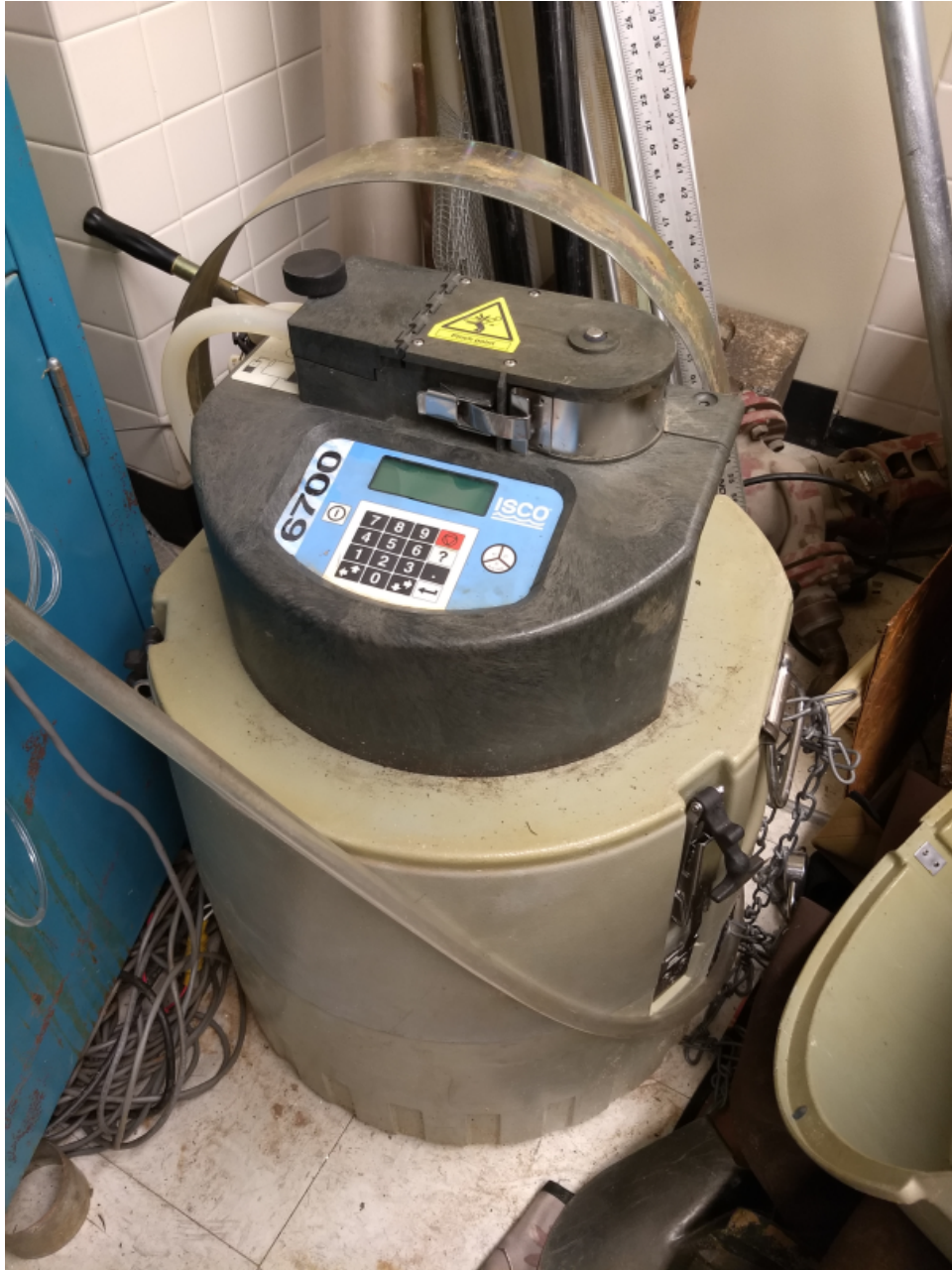
Figure 4.12: Teledyne ISCO 6700 Autosampler used in turbidity and TSS characterization of samples taken from Soapstone Branch during rain events.
