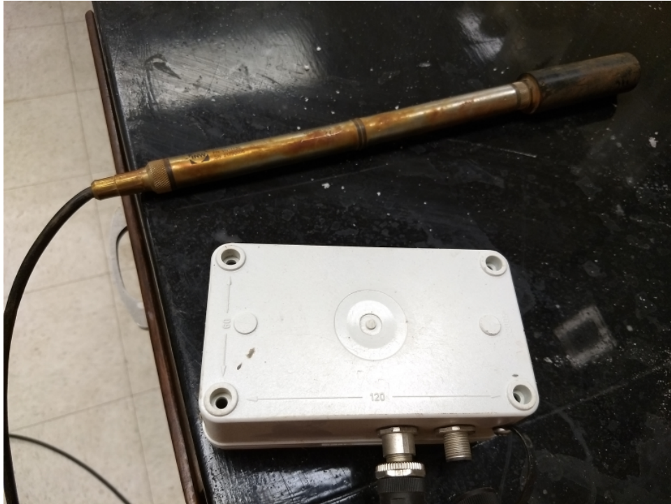
Figure 4.13: INW Turbo turbidity sensor, with logger box, that was used in the Soapstone Branch sediment characterization. Sediment loading covered the sensor head (black), preventing the correct sensor operation.
