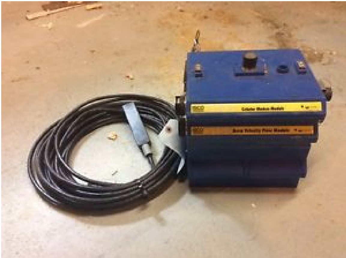
Figure 4.9: Teledyne 2150 AV sensor used in this research, with data acquisition box, battery and connecting cable.
