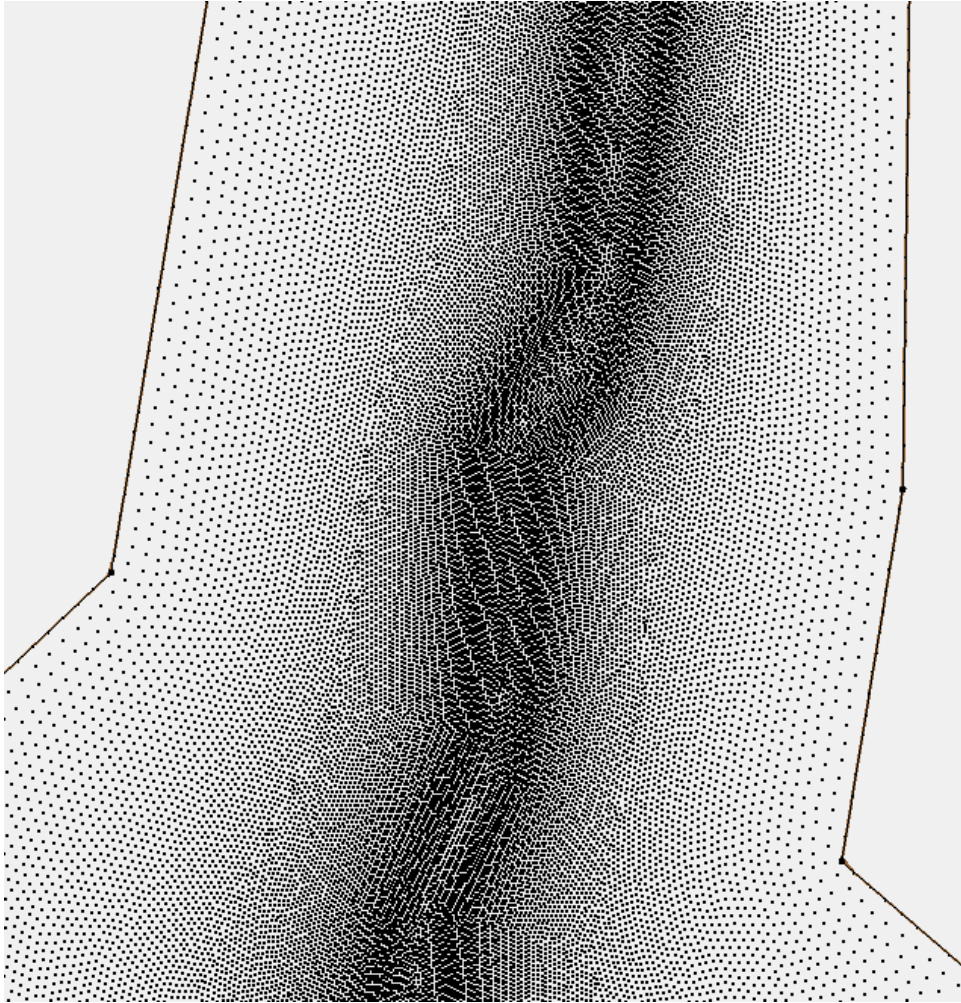
Figure 4.17: Section of the SRH-2D grid points from the mesh generated through SMS, showing how the points are more spaced as it distances from the channel.
