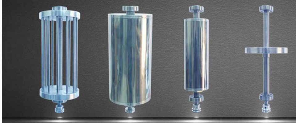
FIGURE 1-5. Variations on the rotating collectors employed in electrospinning process.
