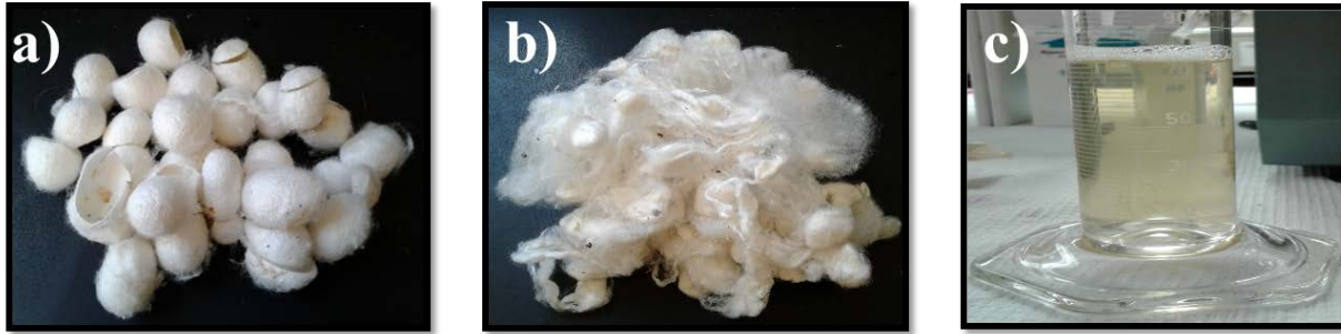
FIGURE 2- 2. Presentation of silk through various steps. a) Partially degummed silk cocoons form industrial waste; b) Degummed silk, c) Regenerated silk fibroin.
