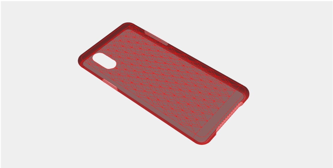
Figure 121: Completed diamond paneling option for phone case
