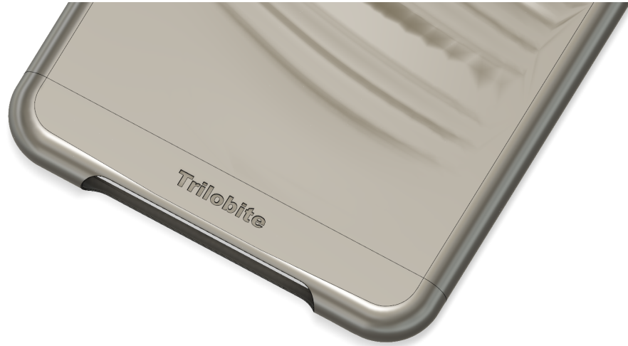
Figure 133: Brand name added from extruded cuts.
