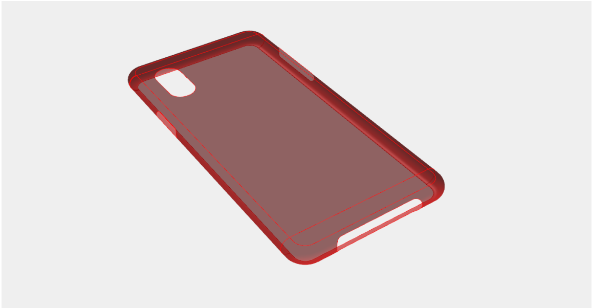
Figure 112: Full algorithmic phone case surface with slots removed
