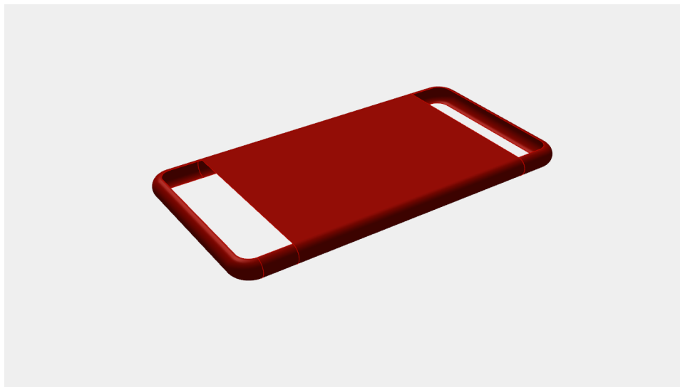
Figure 80: New middle swept surface with end surfaces on the sides
