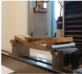
Figure 1.8. OSB sample being tested in the Z010 static material tester
