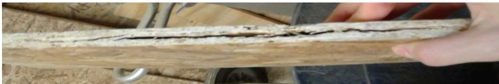
Figure 3.3. Delamination problem in panel
