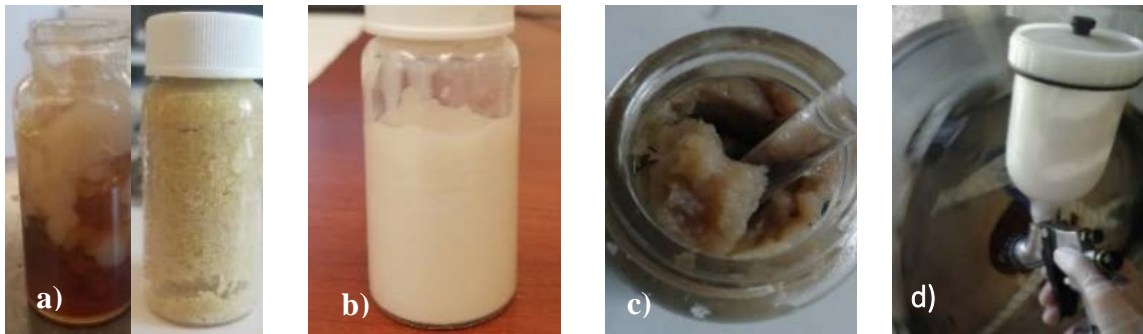
Figure 3.1. a) CNF with pMDI, b) CNF with wax, c) CNF 7 wt. %, d) Not fluid mixture of CNF in wax
