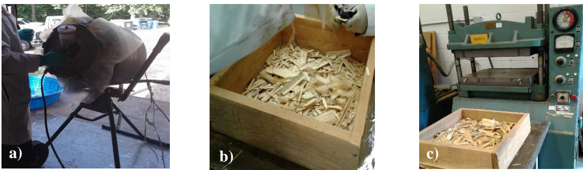
Figure 2.3. a) laboratory blending step b) laboratory forming line c) laboratory pressing step
