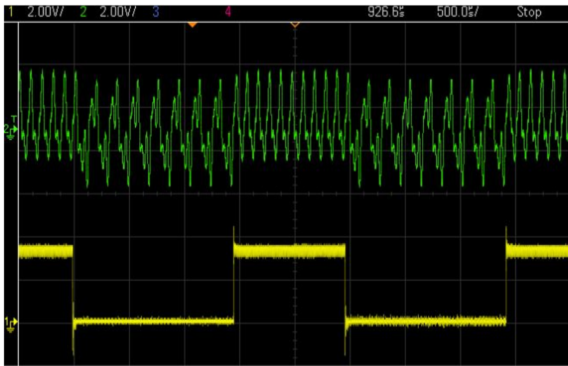
Figure 3.41: Controller input (yellow) and oscillator output given the binary sequence (green). Note the transient periods between oscillator states.
