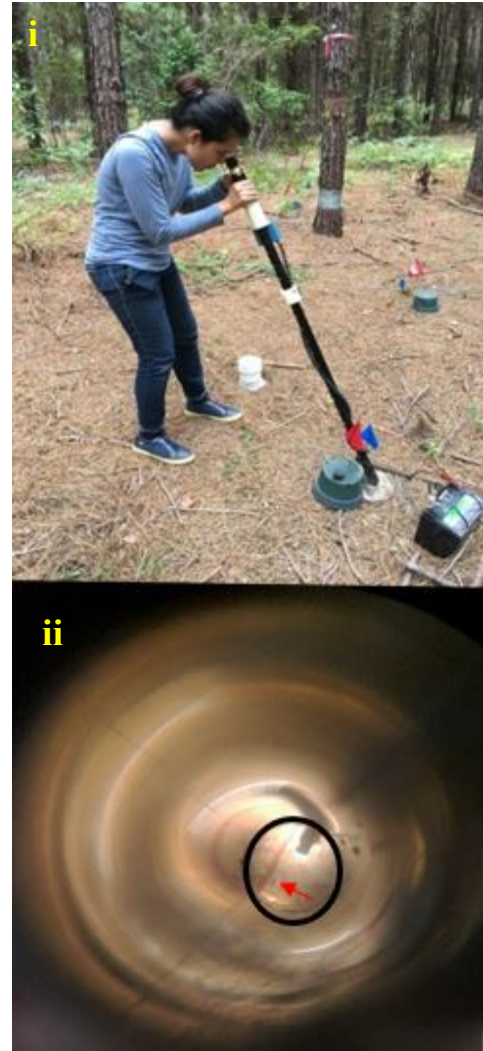
Figure 4.8. (i) Observing root intersections with an optical periscope. The black rectangular object on the ground is a battery which is connected to the periscope to power the light, (ii) the faint line noted by the red arrow is a new root.
