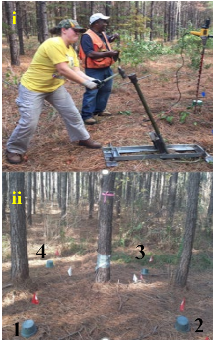
Figure 4.6. (i) Drilling holes using an extension bar and drill bit, (ii) Numbers (1-4) indicate the point where tubes were installed around a single tree.
