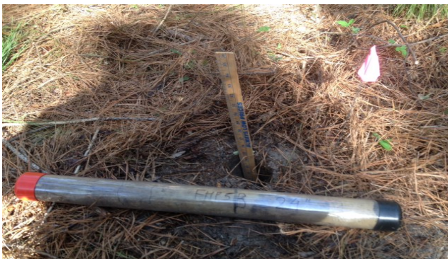
Figure 4.10. Soil core with approximately 50 cm deep soil sample.
