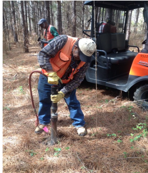
Figure 2.5. Pneumatic soil core sampler with a plastic tube inside it used to collect soil cores.
