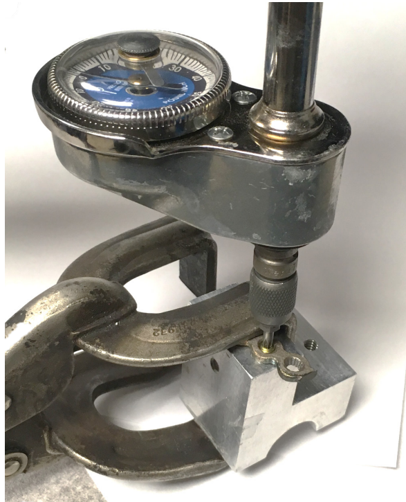
Figure 20: Insertion of the screw using a fixture for angle control and a torque measuring screwdriver.
