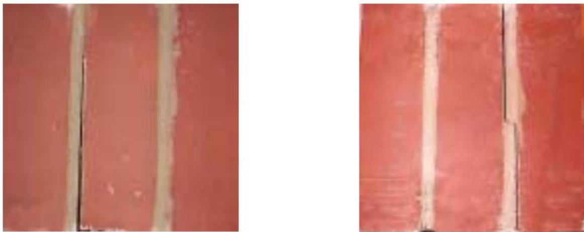
Figure 2-15: Tensile and Shear Bond Failure in Triplet Specimens (Beattie, Molyneaux, et al. 2001)
