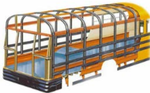
Figure 4.3. School bus roof structure (courtesy of Blue Bird Corporation).
