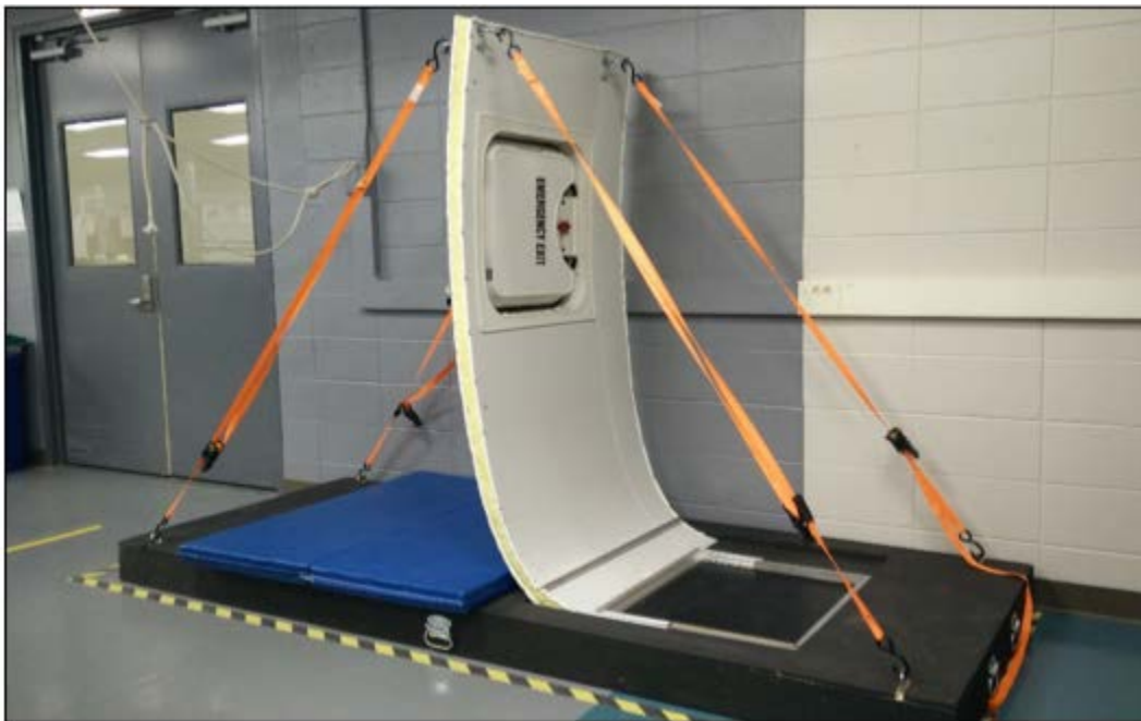
Figure 4.1. Roof hatch test fixture developed by Abulhassan et al. [6].
