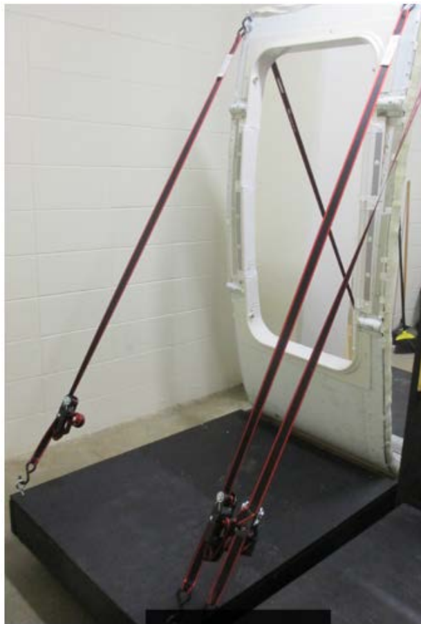
Figure 4.4. Redesigned roof hatch providing a larger opening.
