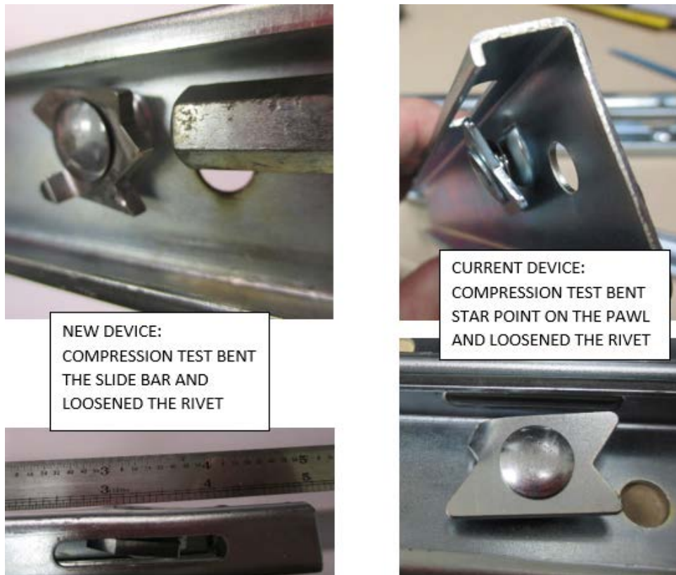
Figure 3.14. Compression test failure modes.
