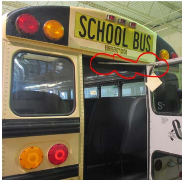
Figure 3.5. Typical rear emergency door hold-open device location.
