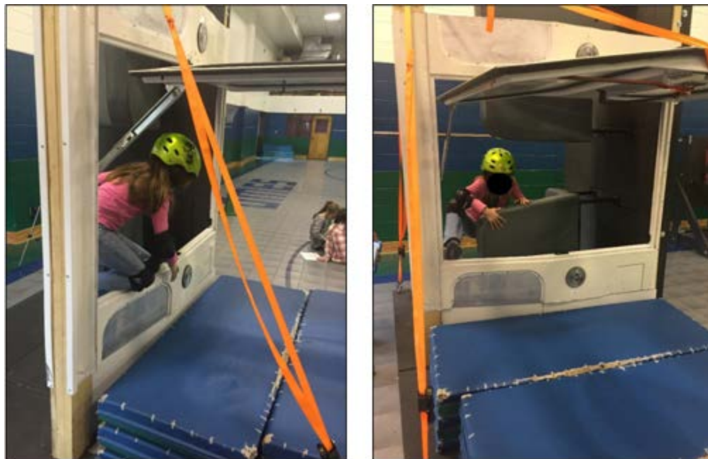
Figure 3.9. Rear emergency exit door with safety mats in place.
