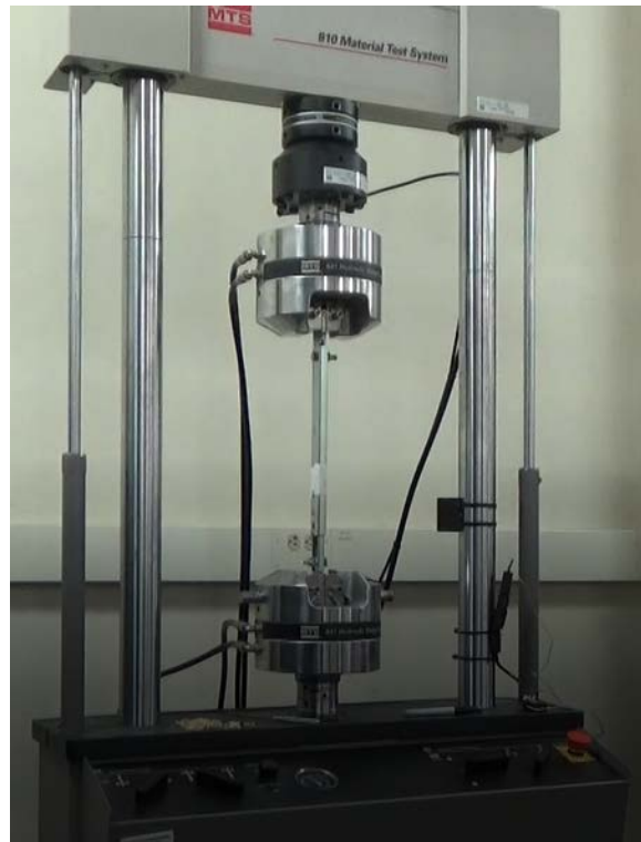
Figure 3.8. Compression testing of door hold-open device.
