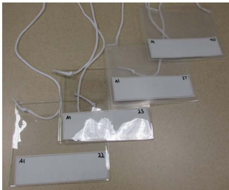
Figure 5.2. RFID tags attached to lanyards.
