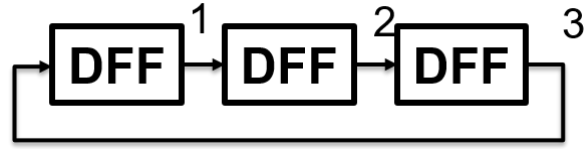
Figure 4.31: Ring counter using D flip-flops.
