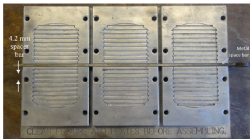
Figure 4.10 Base Plate (TxDOT, 2017)
