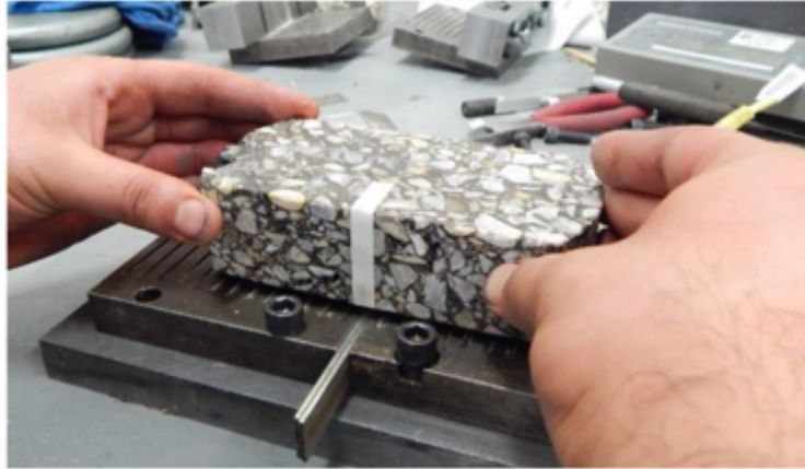
Figure 4.11 Glue and Align the Specimen (TxDOT, 2017)
