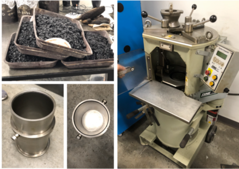
Figure 4.6 Specimen Shaping before Overlay Test
