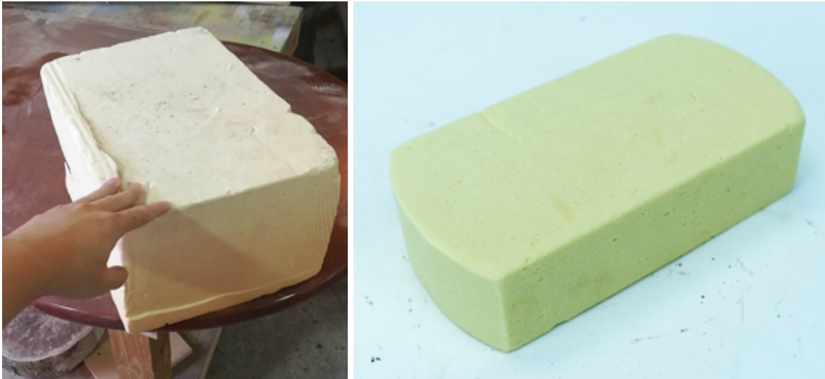
Figure 4.2 A Piece of Polyurethane (Left) and Template Made of Polyurethane Foam (Right)
