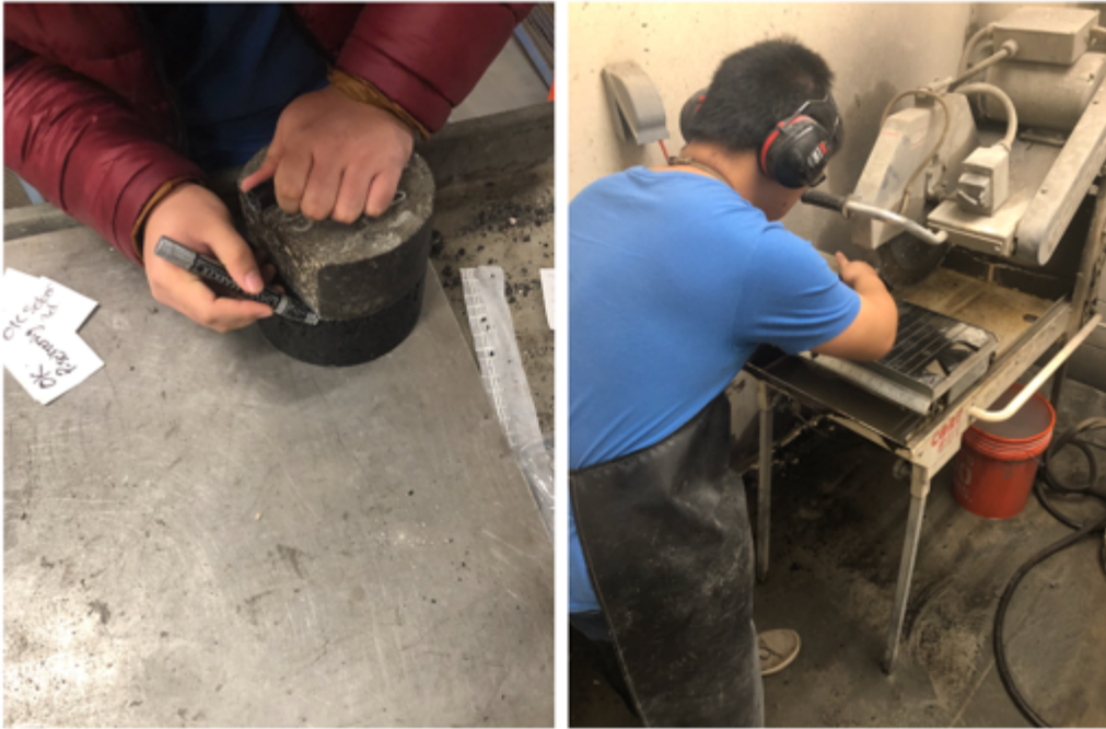
Figure 4.15 Draw Lines and Trimming
