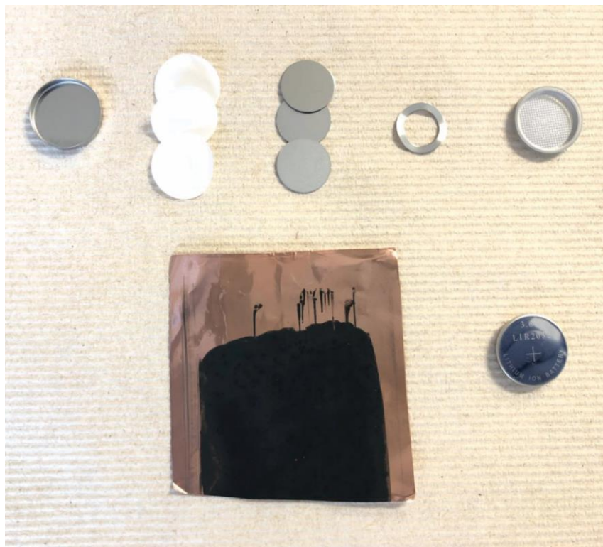
Fig.2.7 The CR-2032 cell assembly components and casted anode material on the copper foil. Celgard separator, wave spring, coin cell cases and an assembled cell are also shown in the image.
