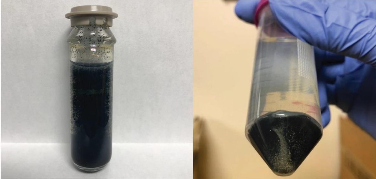
Fig. 2.8 \text{SnO}_x/\text{Ti}_3\text{C}_2\text{T}_x suspension (a) The 10- \text{SnO}_x/\text{Ti}_3\text{C}_2\text{T}_x in microwave container; (b) sediment from 20- \text{SnO}_x/\text{Ti}_3\text{C}_2\text{T}_x after centrifugal in 3500 rpm.
