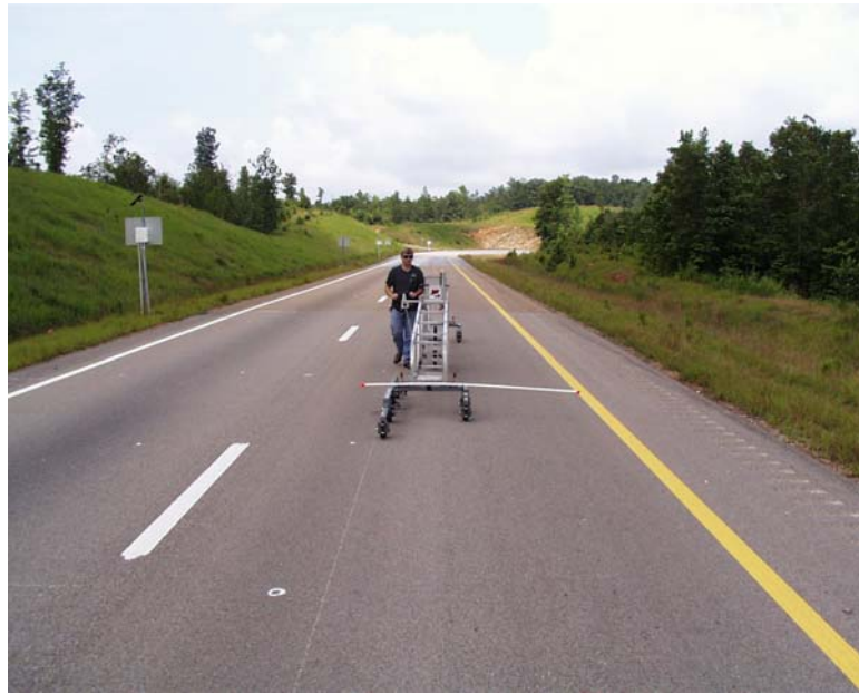
Figure 3-2. McCracken Model Profilograph with guide.
