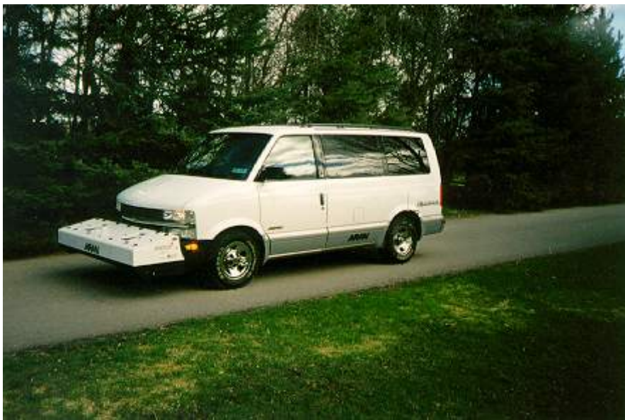
Figure 2-4. Automatic Road Analyzer – ARAN (8).
