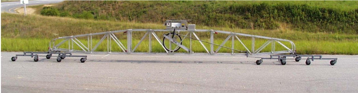
Figure 2-1. McCracken Model California Profilograph.
