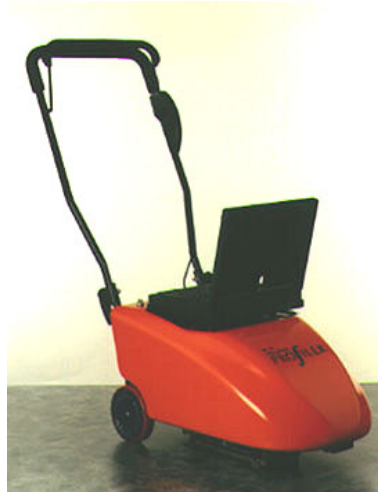
Figure 2-2. ARRB Walking Profiler (5).
