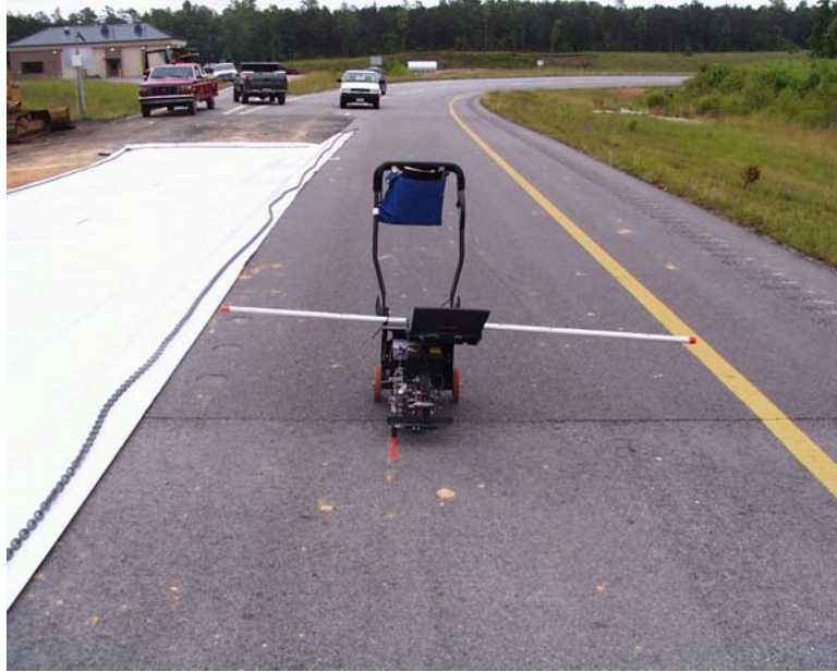
Figure 3-3. ARRB Walking Profiler with guide.
