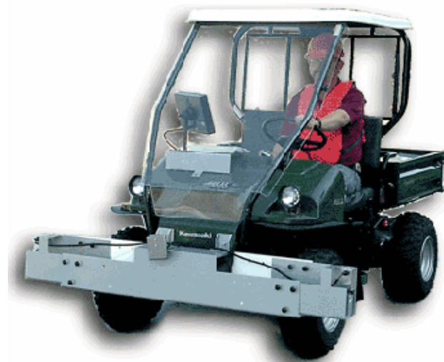
Figure 2-3. ICC Lightweight Inertial Profiler (7).
