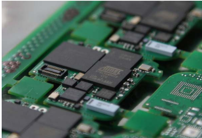
Figure 1-6: Surface Mount Technology [15]
