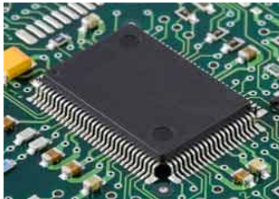
Figure 1-7: Quad Flat Package [17]
