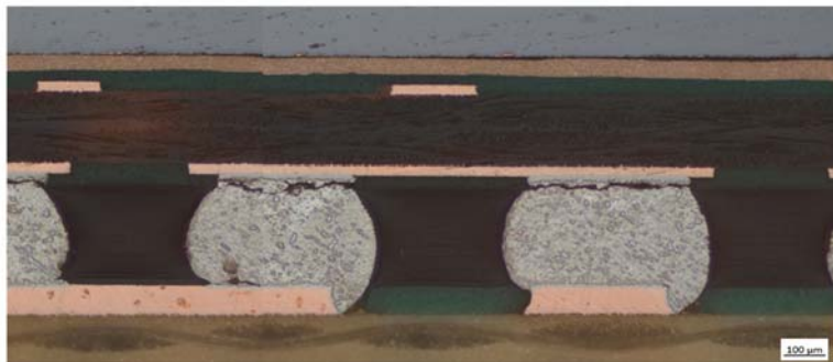
Figure 5-4: TC1 SAC305 and TC2 Inventec CABGA208 Cross Sections 12m [37]
