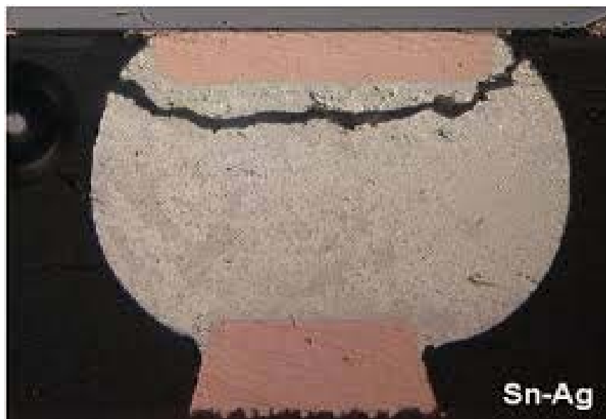
Figure 3-3: Crack Through Solder [90]
