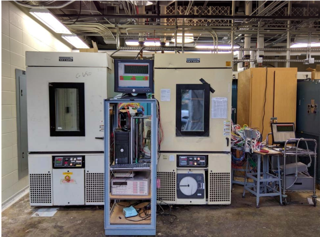
Figure 4-6: Thermal Cycling Chambers [93]
