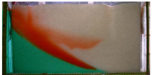
Figure 5.3: Photographs of the beach face infiltration (Source 1) and open well injection (Source 2) experiment
