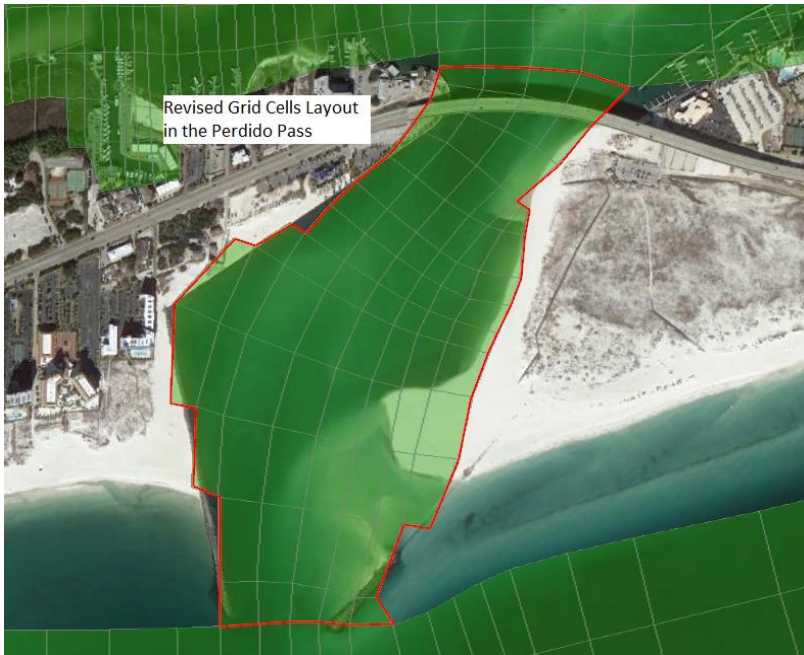
Figure 3-5 Grid cells layout comparison between original and revised scenarios in the Perdido Pass
