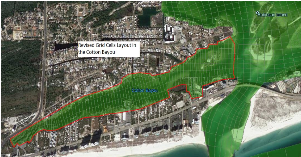
Figure 3-6 Grid cells layout comparison between original and revised scenarios in the Cotton Bayou
