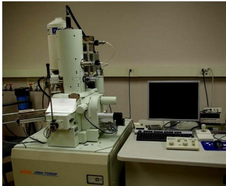
Figure 2.4: The JEOL JSM 7000F FE-SEM Scanning Electron Microscopy (SEM) used in the microstructure determination of composites.
