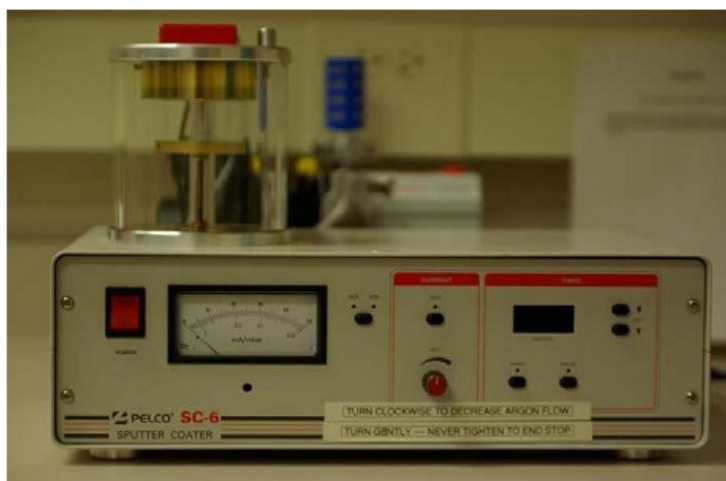
Figure 2.5: The Pelco SC-6 sputter used for gold coating.
