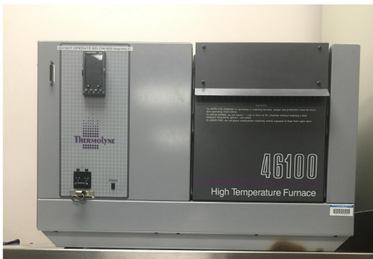
Figure 2.2: Image of 46100 Barnstead Thermolyne furnace.
