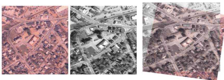
Figure 3.2: Different views aerial images registration to extend the view. (This image is from MathWorks website Image Registration section, and the link is https://www.mathworks.com/discovery/image-registration.html )
