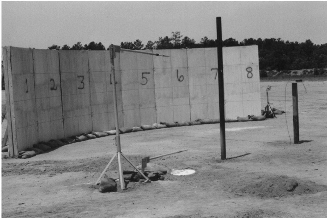
Figure 11. FRAT eight screen configuration demonstration, from Barnard and Nebolsine [5].
