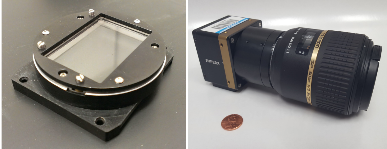
Figure 4. Photo of the microlens array in the custom mount designed by the AFDL (left) and photo of the plenoptic camera constructed by the AFDL equipped with a 60 mm Tamron main lens (right).
