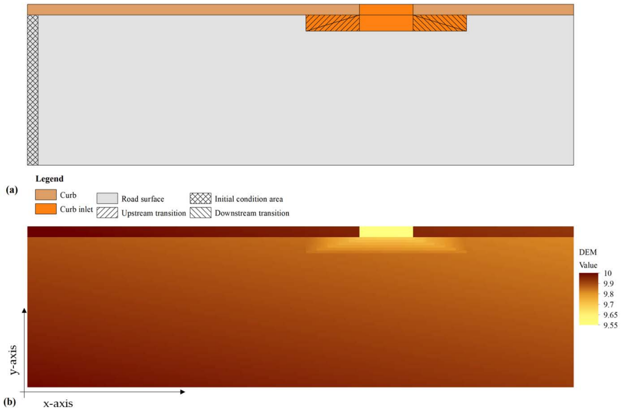
Figure 4.3. (a) Layout of type C curb inlet evaluation experiment (top view), and (b) DEM of case C01 with a longitudinal slope, S_0 = 0.004 , and cross slope, S_x = 0.0208 .
