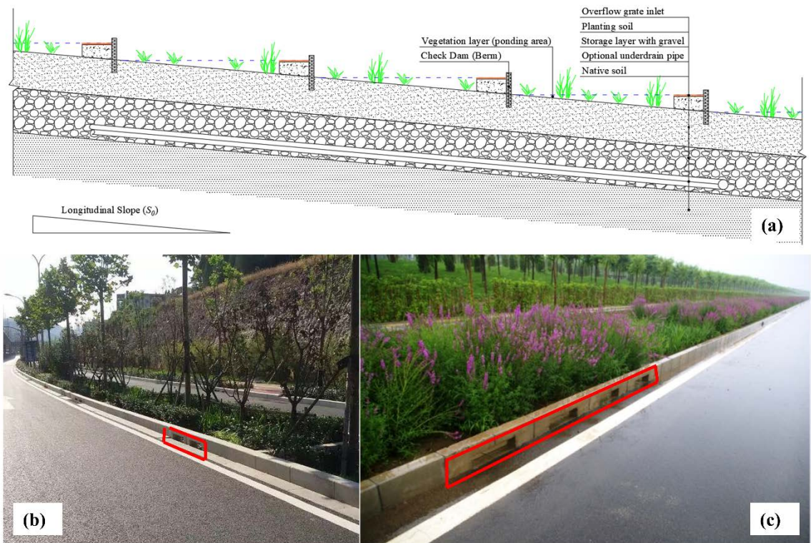
Figure 1.1. (a) Schematic diagram of a continuous road-bioretenion strip. (b) and (c) road-bioretenion strips constructed in China with red box showing the curb inlet.
