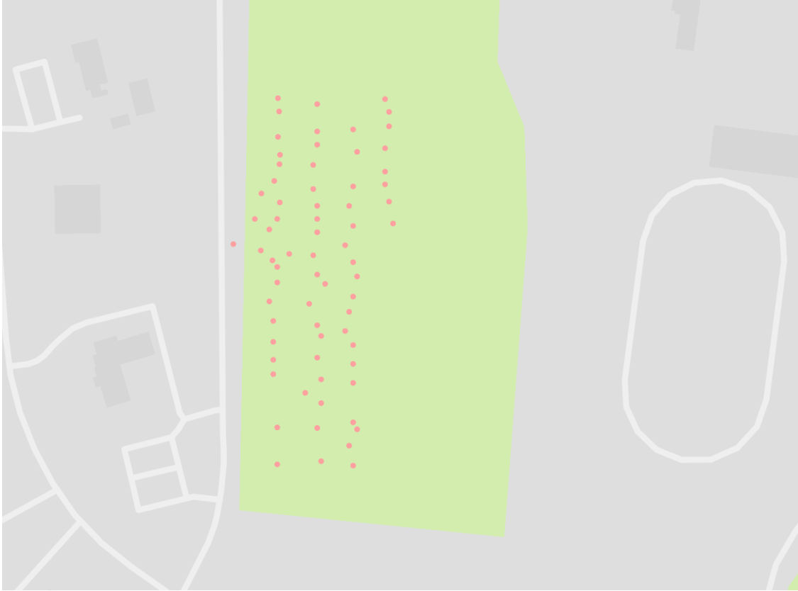
Figure 6.10: Test of 80 Coherent eMotes with Reported GPS Positions Mapped
