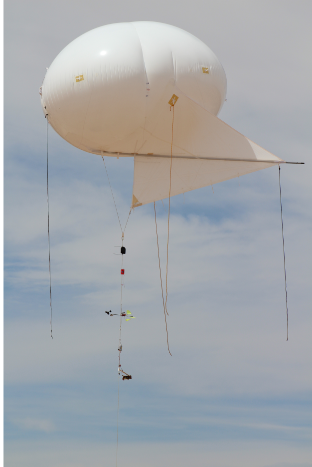
Figure 6.13: Balloon with Tethered eMotes and Reference Sensors
